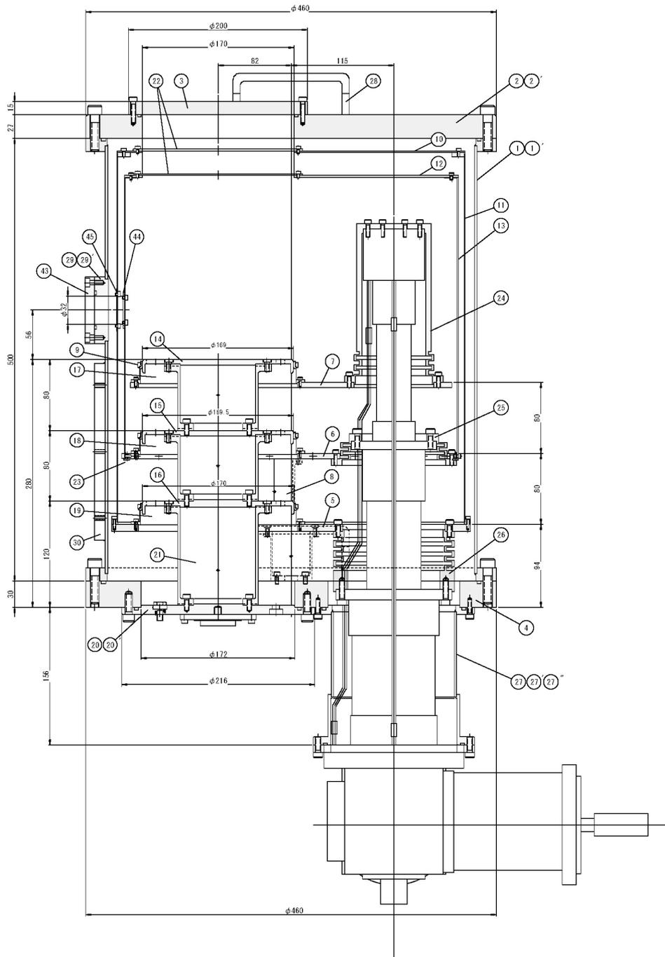
Figure 2: A cross-sectional view of the cartridge-type cryostat. The cryostat is composed of 3 stages, 4 K, 12 K, and 80 K from up to own. The parts number is indicated.
