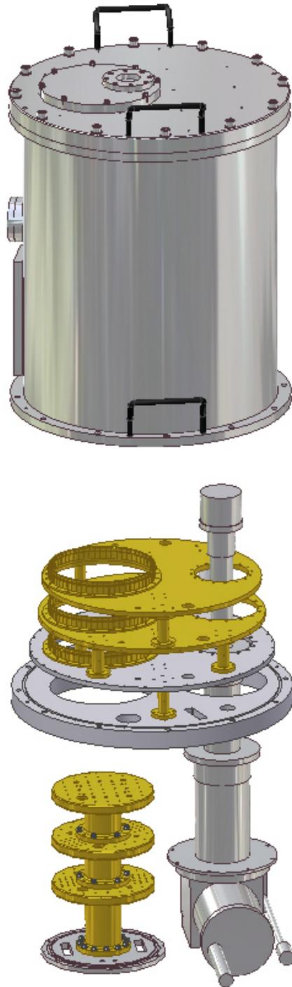
Figure 1: Schematic drawing of the cartridge test cryostat. There are three plates of 4 K, 12 K, and 80 K from up to down.
