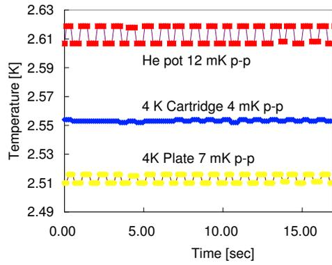
Figure 9: The temperature variation on the 4 K stage and plate in 20 seconds. The ripple is associated with the cold head displacement of 3 stage GM cryocooler.
