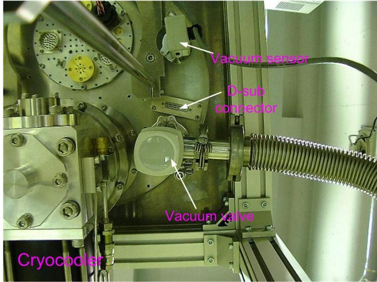
Figure 7: The bottom plate of the cryostat.
