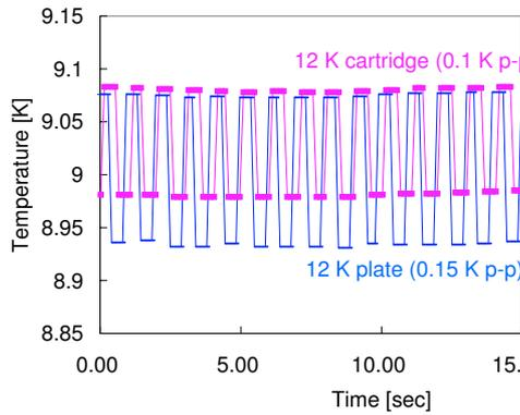
Figure 10: The temperature variation on the 12 K stage and plate in 20 seconds. The ripple is associated with the cold head displacement of 3 stage GM cryocooler.
