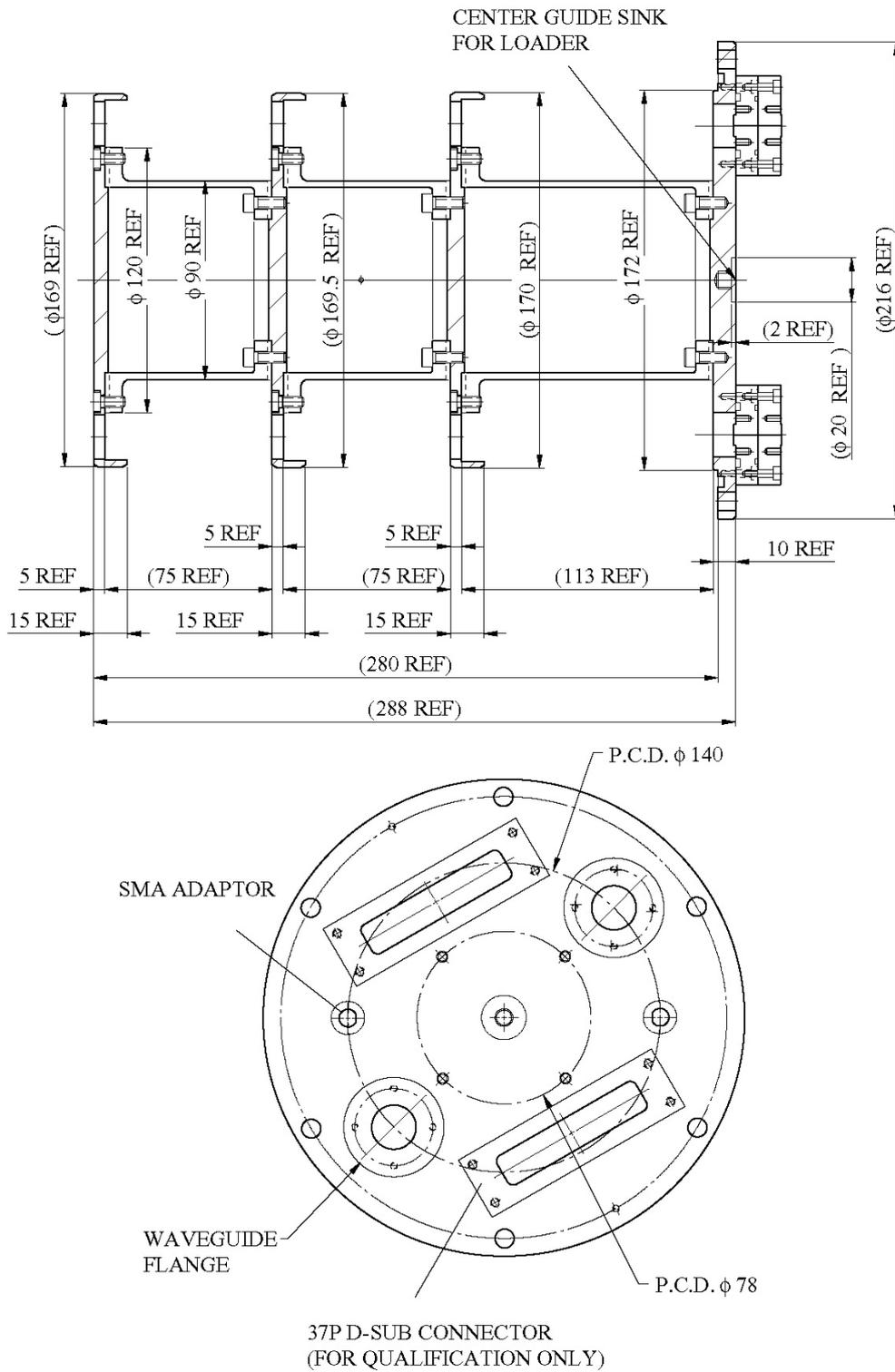
Figure 3: A schematic drawing of the cartridge structure.
