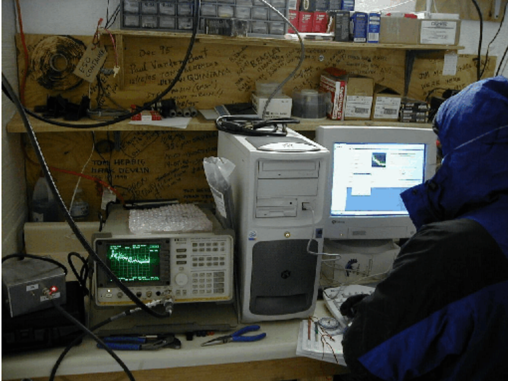
Figure 4: Spectrum analyzer and data collection software. Note bias tee providing 15 VDC to preamps via the RF cable.
