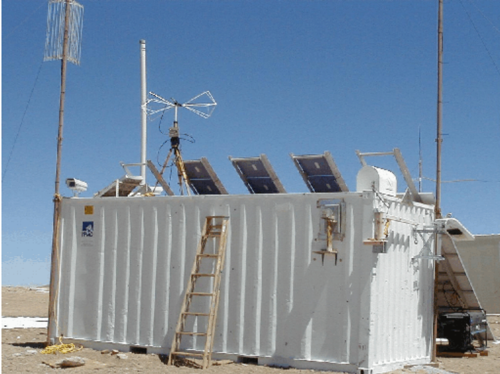
Figure 2: NRAO instrument container at Chajnantor with the biconical antenna for the RFI survey.
