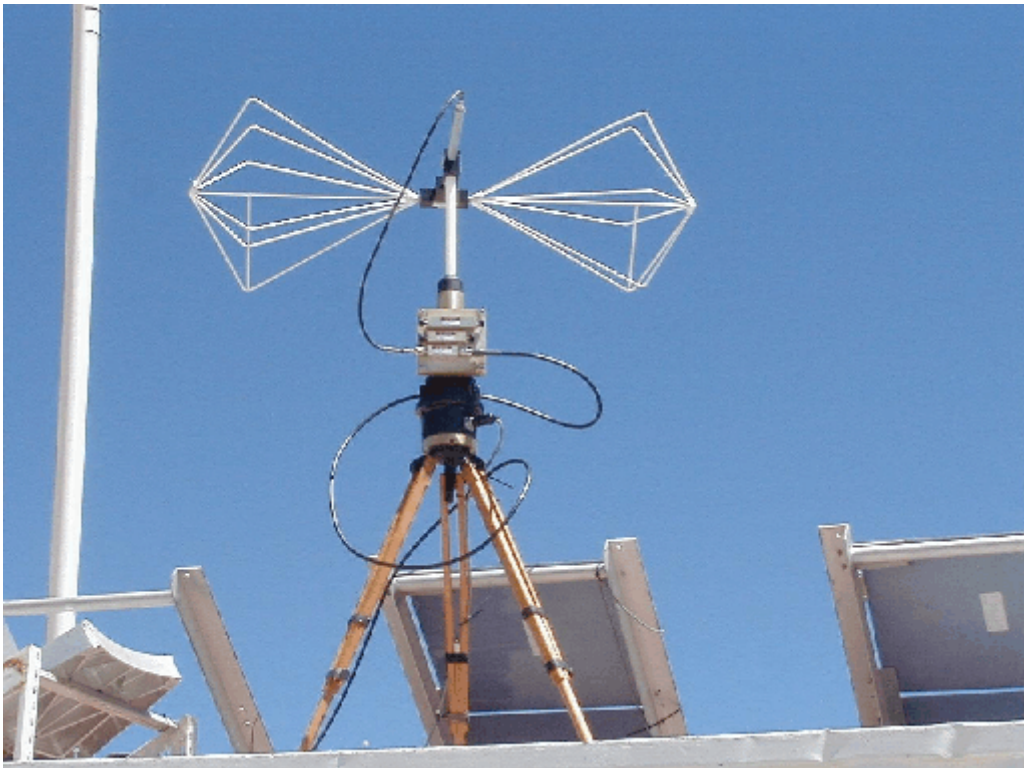
Figure 3: Biconical antenna with preamps, rotor, and tripod.
