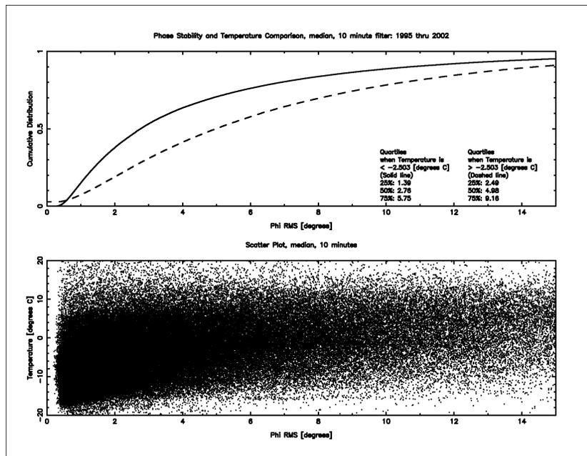
Figure 10: Cumulative distributions of the maximum 11.2 GHz phase fluctuations measured at Chajnantor when the temperature was above or below the median.
