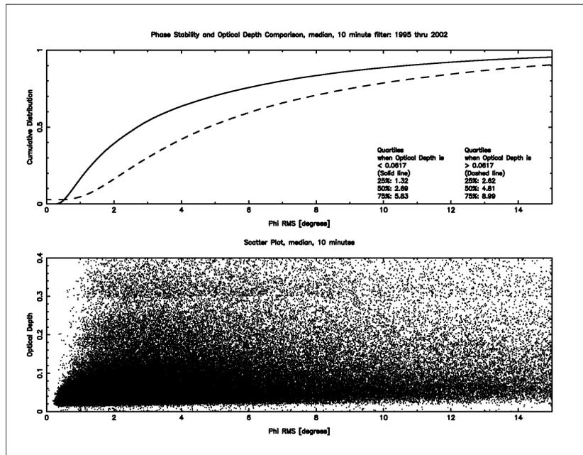
Figure 11: Cumulative distributions of the maximum 11.2 GHz phase fluctuations measured at Chajnantor when the 225 GHz zenith optical depth ( $\tau_{225}$ ) was above or below the median.
