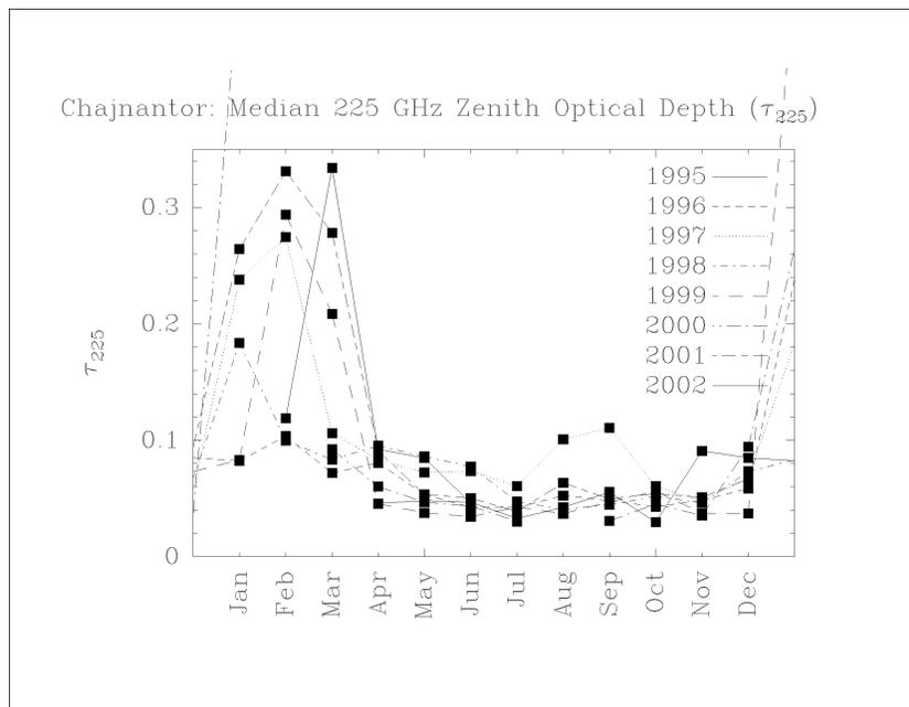
Figure 2: Seasonal variation of median measured 225 GHz zenith optical depths at Chajnantor. The variation of the broadband  $350\mu\text{m}$  measurements is similar.
