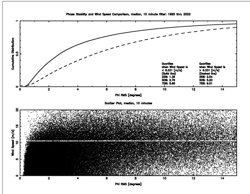
Figure 9: Cumulative distributions of the maximum 11.2 GHz phase fluctuations measured at Chajnantor when the wind speed was above or below the median.
