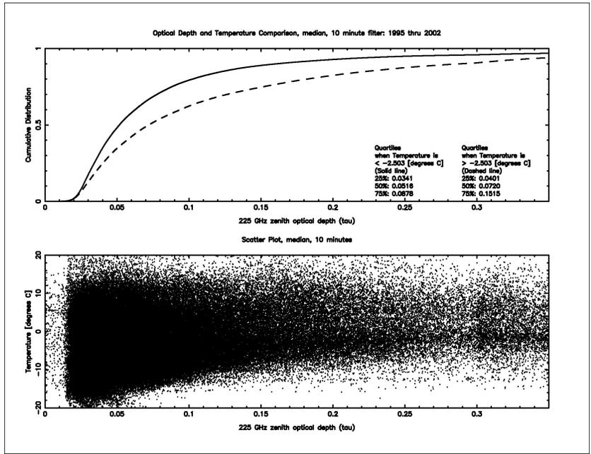
Figure 7: Cumulative distributions of the 225 GHz zenith optical depths ( $\tau_{225}$ ) measured at Chajnantor when the temperature was above or below the median.
