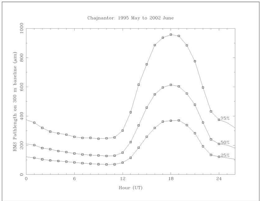
Figure 5: Diurnal variation of quartiles of measured phase fluctuations at Chajnantor referred to the zenith.
