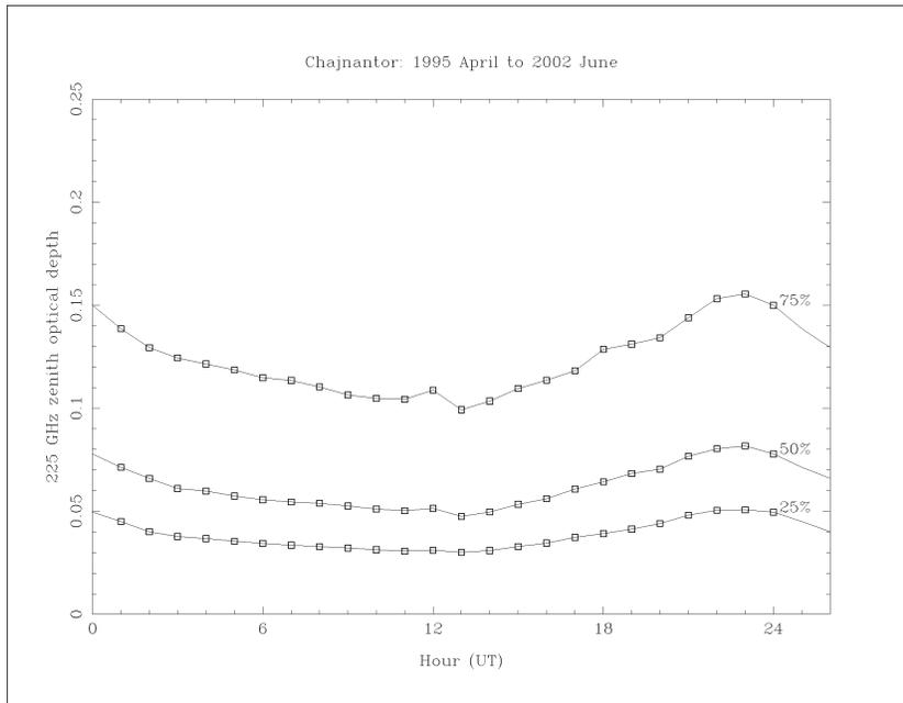
Figure 3: Diurnal variation of quartiles of measured 225 GHz zenith optical depths at Chajnantor. Local solar time is  $UT - 4^h 31^m$ . The variation of the broadband  $350\mu m$  measurements is similar.
