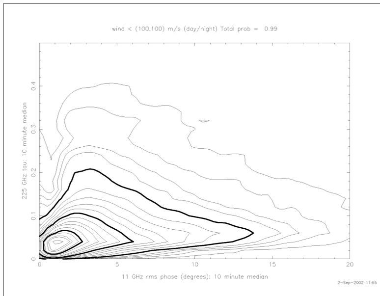
Figure 15: Joint probability distribution of  $\tau(225)$  and  $\phi(rms)$  with a very loose wind (pointing) requirement: that the wind speed be less than 100 m/s either day or night. The contours encircle 5, 10, 15, ... per cent of the total probability (99% in this case).
