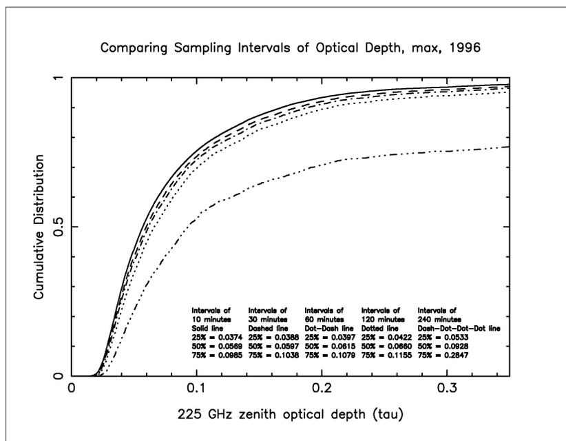
Figure 13: Cumulative distributions of the maximum 225 GHz zenith optical depths ( $\tau_{225}$ ) measured at Chajnantor in 1996 for different sampling intervals. The 240 min interval suffers from a processing defect.
