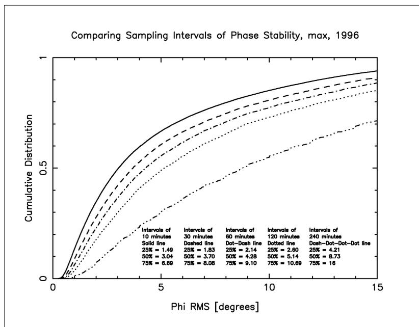
Figure 14: Cumulative distributions of the maximum 11.2 GHz phase fluctuations measured at Chajnantor in 1996 for different sampling intervals. The 240 min interval suffers from a processing defect.
