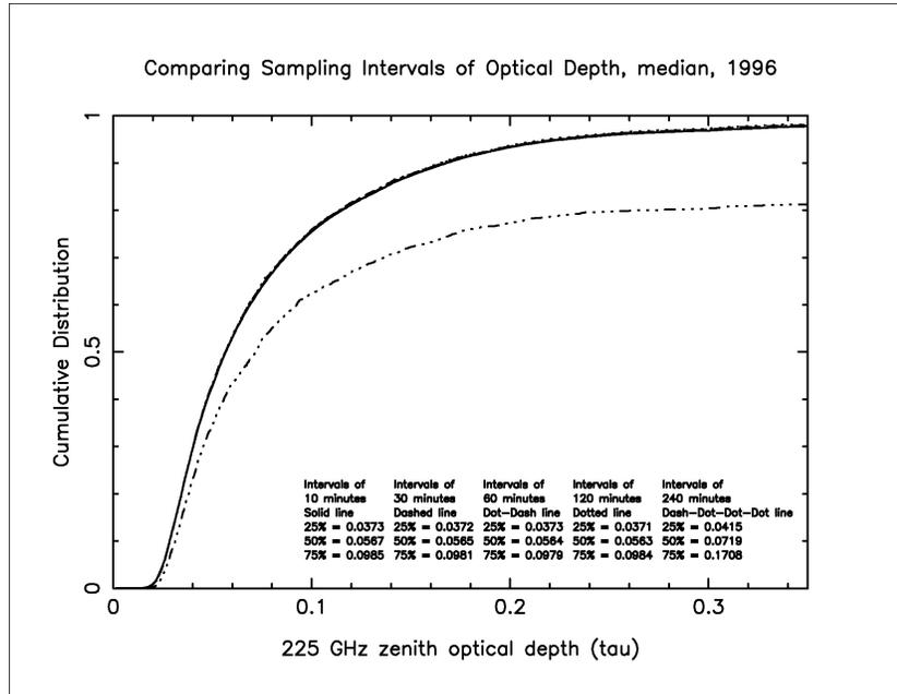
Figure 12: Cumulative distributions of the median 225 GHz zenith optical depths ( $\tau_{225}$ ) measured at Chajnantor in 1996 for different sampling intervals. The 240 min interval suffers from a processing defect.
