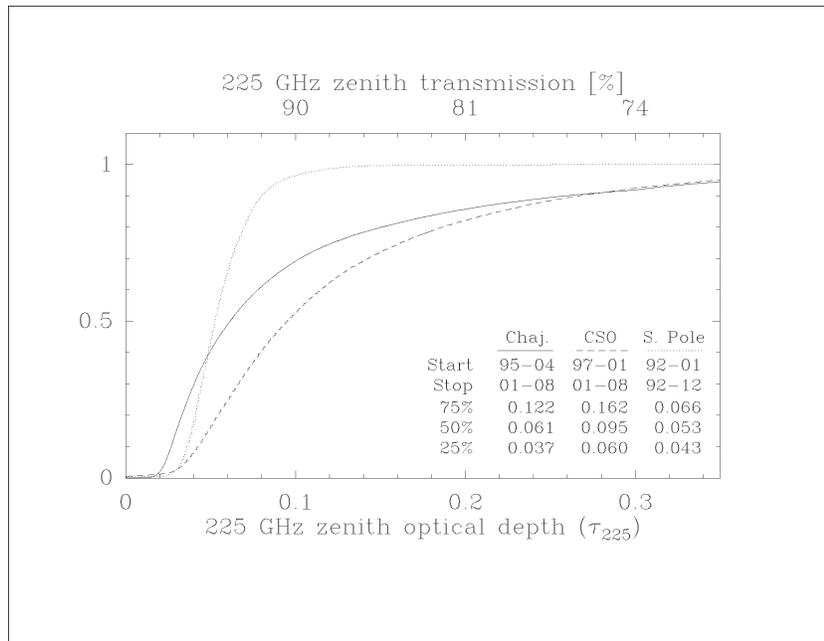
Figure 1: Cumulative distributions of the 225 GHz zenith optical depths ( $\tau_{225}$ ) measured at Chajnantor, at Mauna Kea (CSO), and at the South Pole. Adapted from Radford & Chamberlin (2000). The distributions of the broadband  $350\mu\text{m}$  measurements are similar.
