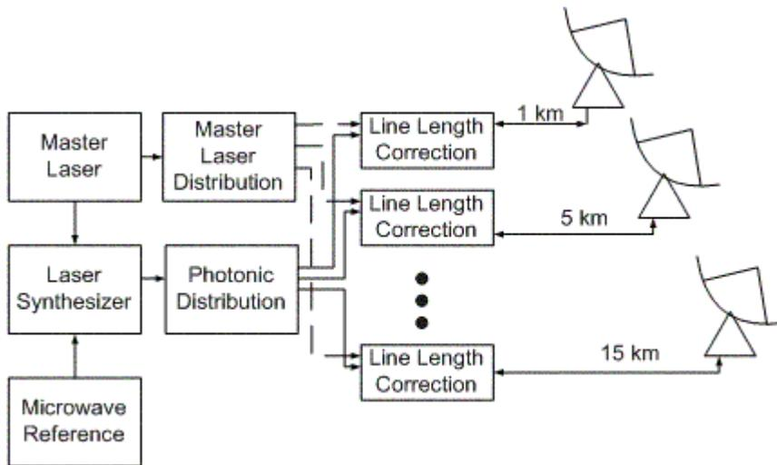
**Figure 1 – System level schematic of the ALMA LO reference generation and distribution.**
