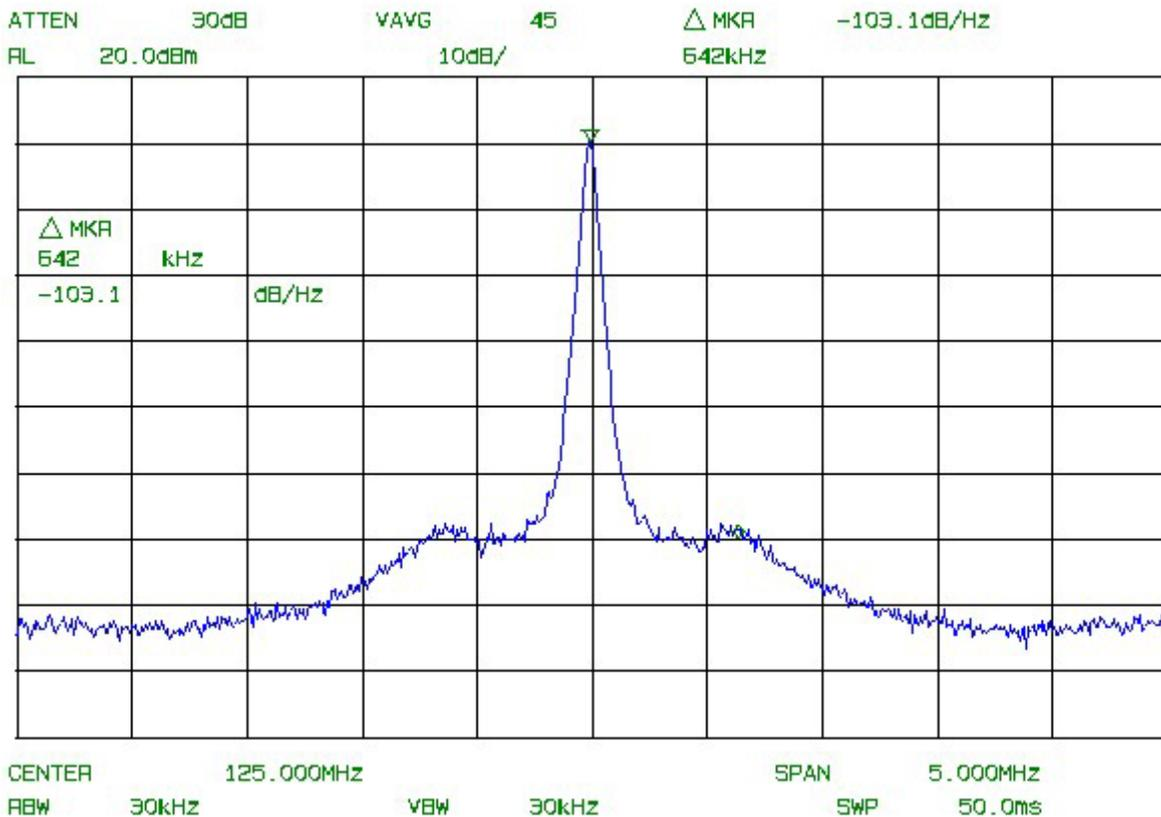
**Figure 5 – Laser Synthesizer Loop IF. Scale is 10 dB/div, RBW=30 kHz, noise marker at 542 kHz offset is -103.1 dBc/Hz**
