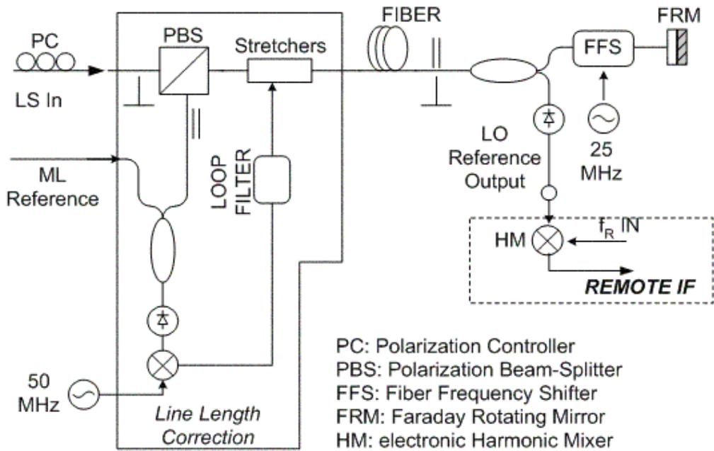
**Figure 6 – Line length correction schematic, showing both central and antenna components, along with items used in the laboratory tests.**
