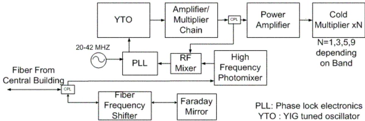
**Figure 2 – LO equipment an antenna, typical. A separate assembly of this type is provided for each band. The reference signal is optically switched to the one in use. An optical amplifier is expected to be required between the coupler and the photomixer but it was not included in the tests presented in this memo.**
