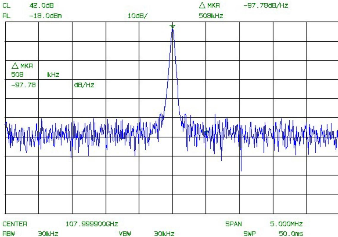
**Figure 4 – Laser Synthesizer Output at 108 GHz (after photomixer). The measurement noise floor -97 dBc/Hz limits the measurement above 200 kHz offset. CF=108 GHz, Span=5 MHz, RBW=30 kHz**
