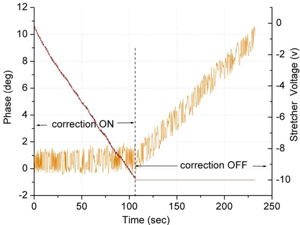
**Figure 7 – Plot of the phase drift of 18.6 GHz signal through 10 km of fiber.**
