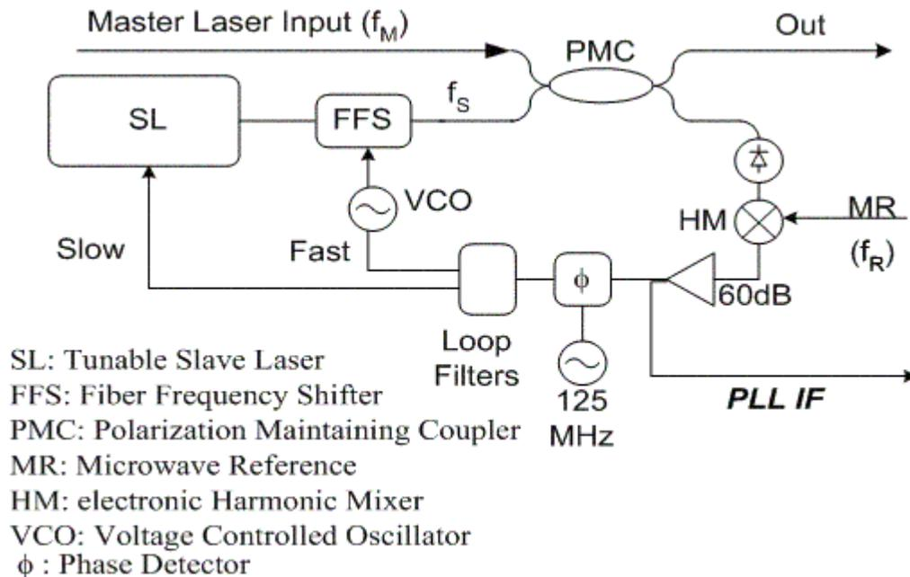
**Figure 3 – Schematic of the laser synthesizer.**
