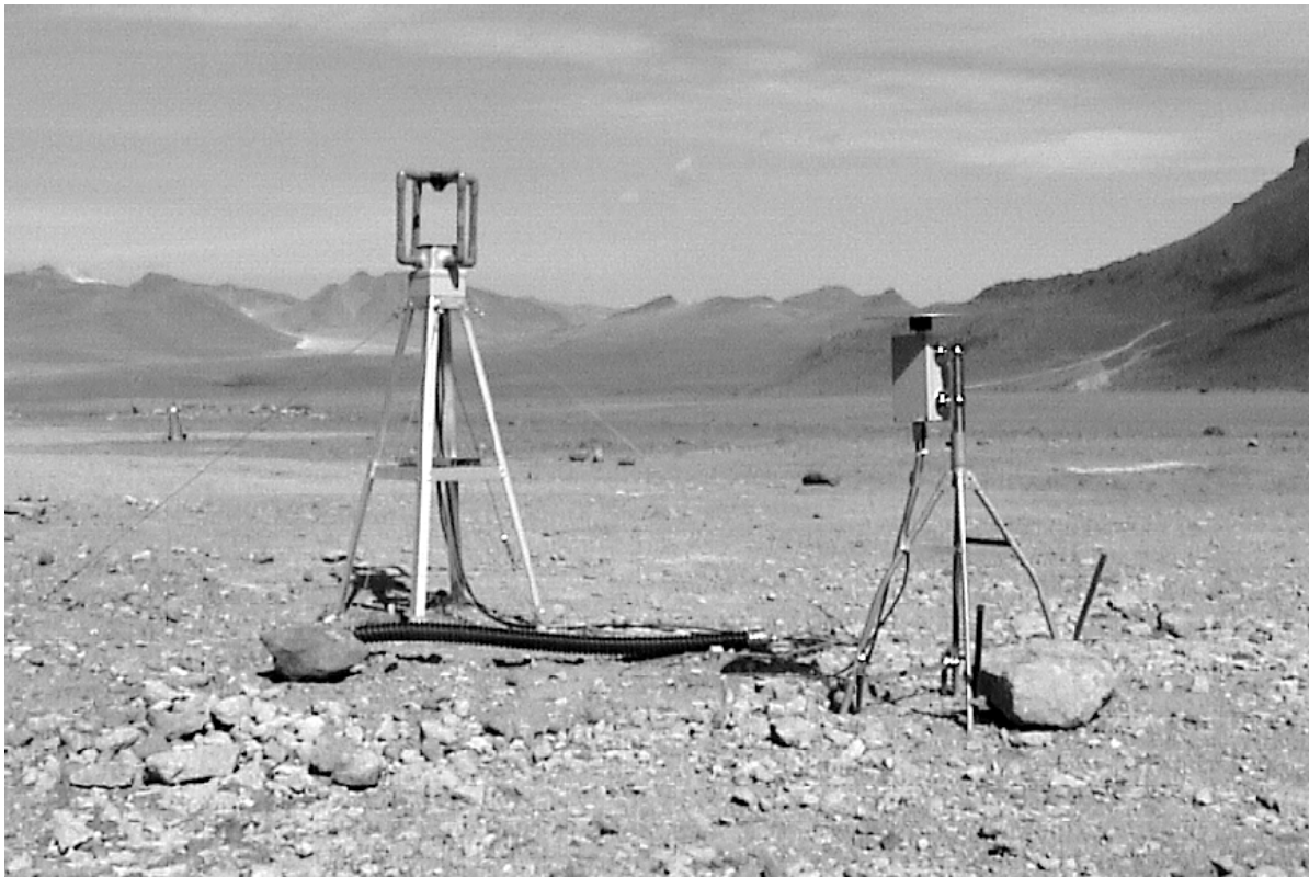
Figure 1: Appearance of the magnetic field antenna ( left ) and the electric field slow antenna ( right ) installed at the site.
