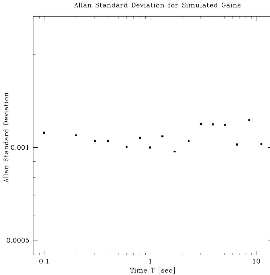
Figure 9: The Allan standard deviation (ie, square root of the Allan variance) for a typical gain series with  $1e-3$  fractional fluctuations at 1 s. As expected for  $1/f$  noise, the Allan standard deviation as a function of integration time is flat.
