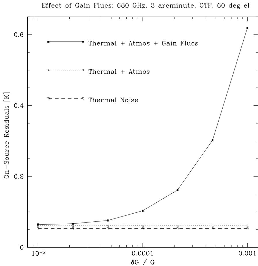
Figure 11: Results of OTF simulations for 680 GHz with 1/f gain fluctuations. Again, the story is gain fluctuations of 1e-4 are OK, and gain fluctuations of 1e-3 are really really bad.
