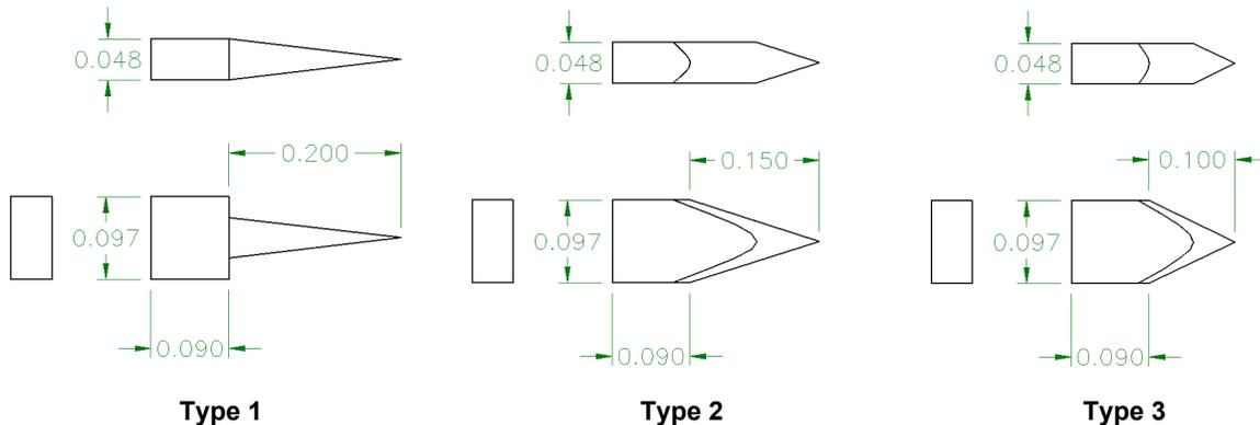
Fig. 1. Three compact waveguide loads. The dimensions, in inches, are for WR-10 waveguide, but they can be scaled to any band.
