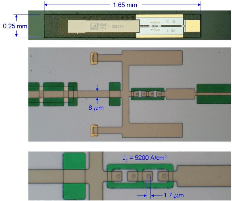
Fig. 5. The SIS mixer substrate.
