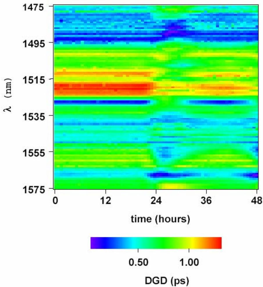
Figure 3 DGD measurement of a low PMD fibre link over time
