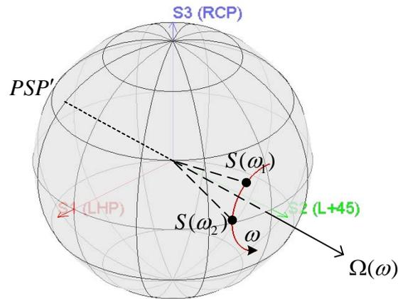
Figure 2 Illustration of PMD Vector on a Poincare Sphere
