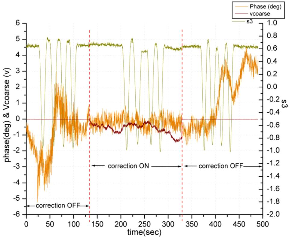
**Figure 25:** 5 Km with twisting  $\frac{1}{2}$  inch of fiber from 0 to  $+ 360$  deg and then back from  $+360$  to 0 deg . The correction is OFF from 0 to 130 sec, then the correction is ON from 125 sec to 327sec, and finally correction is OFF from 327sec to 490 sec.
