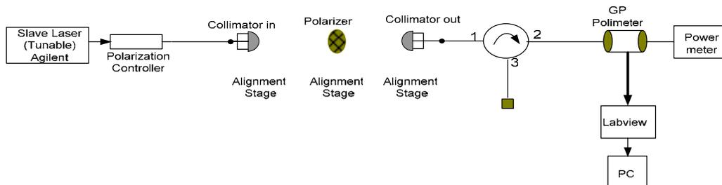
**Figure 3:** Test setup for measuring State-of-Polarization-Dispersion of the optical circulator
