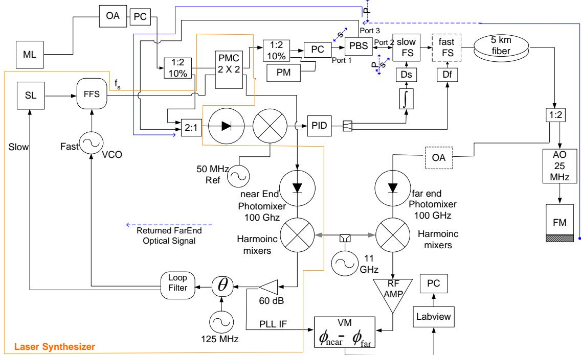
**Figure 30:** Schematic of the Line length correction at 108 GHz reference
