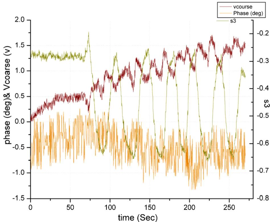
**Figure 22:** 5 km correction is ON all the time. From 0 to 75 sec the fiber is not moving (or bent). From 75 to 270 the fiber is bent multiple times, the bend radius was changing from 2.5 inch to 26 inch
