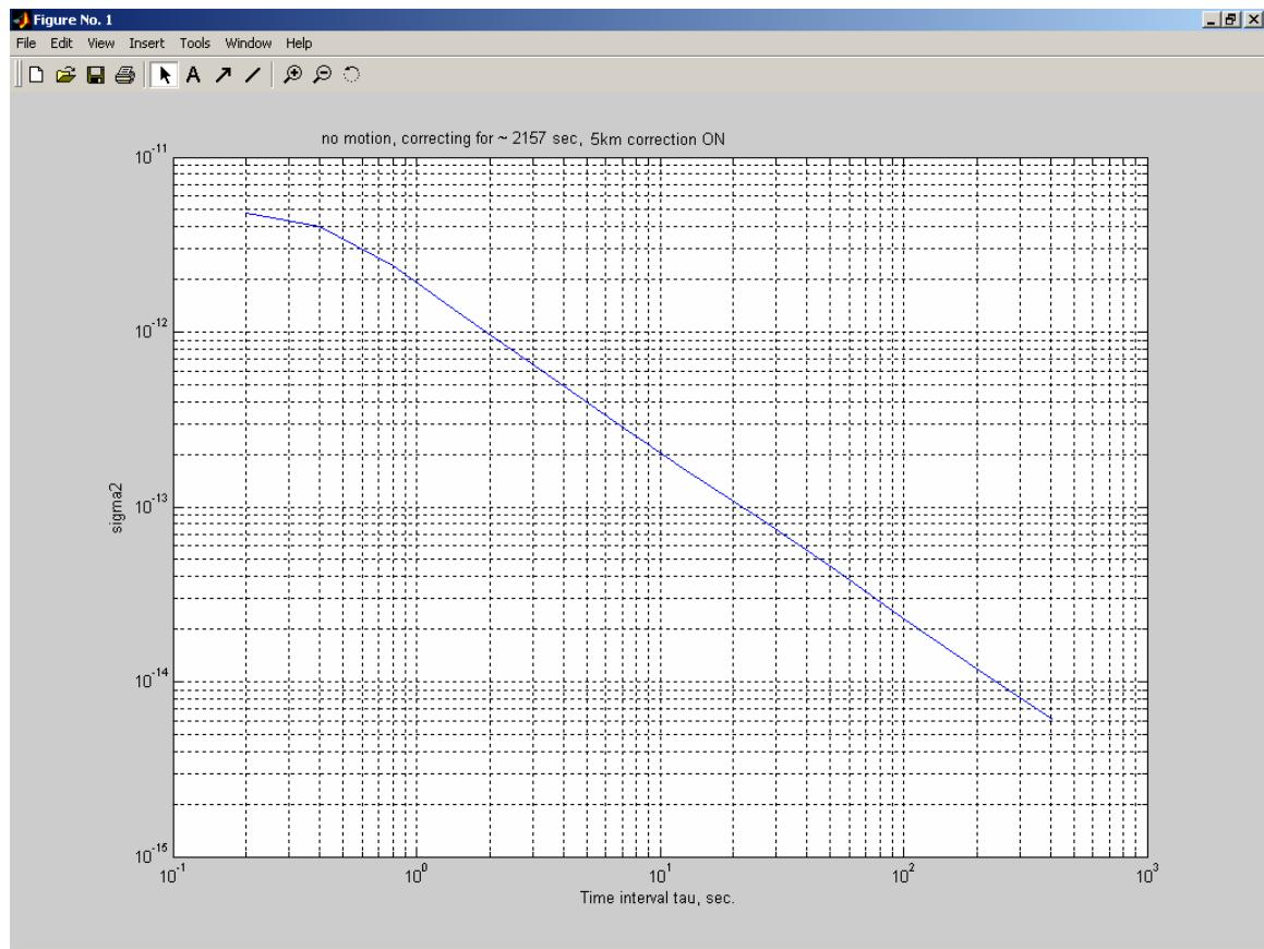
**Figure 17:** the measurement of the Allan variance of the phase in figure 16(5 km fiber length ), for a reference frequency of 20 GHz and sampling time of 0.2 sec.
