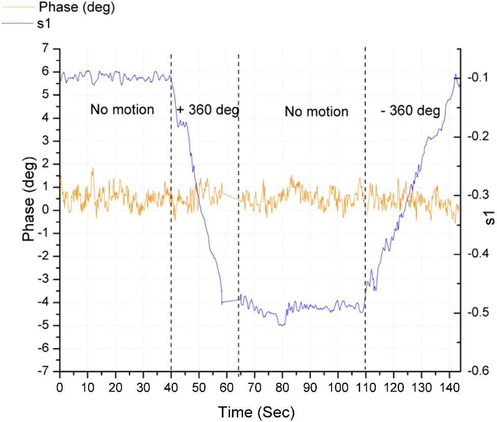
**Figure 7:** Results of test setup Figure #6 The phase fluctuation resulted by moving the fiber by +360 azimuth rotation and back by -360 deg while recording the change in the polarization due to the fiber move. The Master and slave lasers are fully aligned in this test results.
