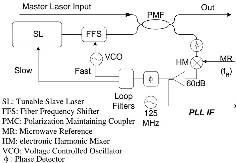
**Figure 29** Schematic of the laser synthesizer.
