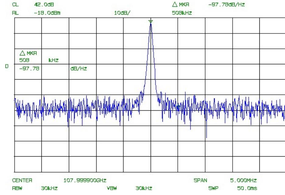
**Figure 31:** Laser Synthesizer Output at 108 GHz (after photomixer). The measurement noise floor at -97 dBc/Hz limits the measurement above 200 kHz.
