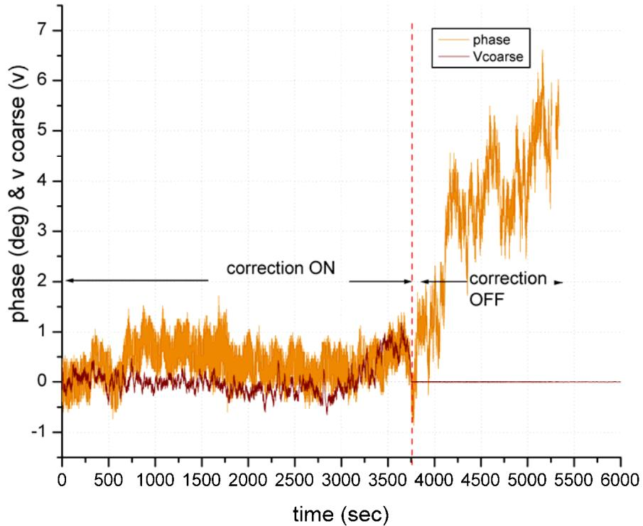
**Figure 13:** Plot of phase drift for a baseline test in which 1-m of fiber is inserted between the stretcher and the far end without using an OA at the far-end (Fig. 12).
