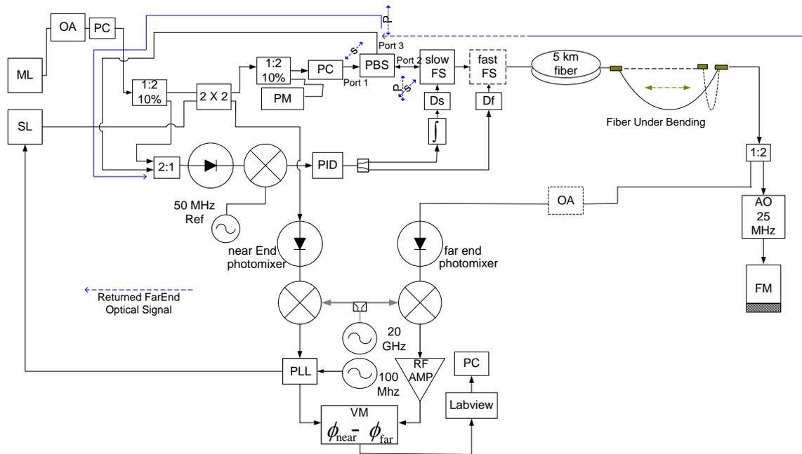
**Figure 12 - Farady Mirror** test setup for the line length correction system without the use of an optical circulator. Instead we used the combination of PBS and faraday mirror to rout the light signal back to the near end as shown in the blue line
