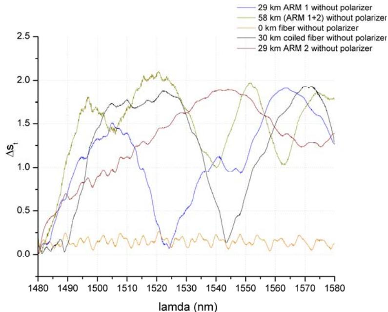
**Figure 9:** Relative polarization change (from initial value) for various fibers-under-test as wavelength is scanned from 1480 to 1580 nm. The vertical axis is  $S_T$  -see Eq(1).
