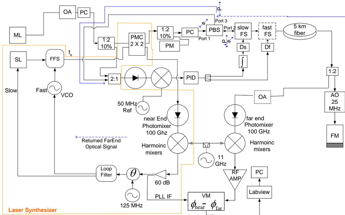
**Figure 30:** Schematic of the Line length correction at 108 GHz reference
