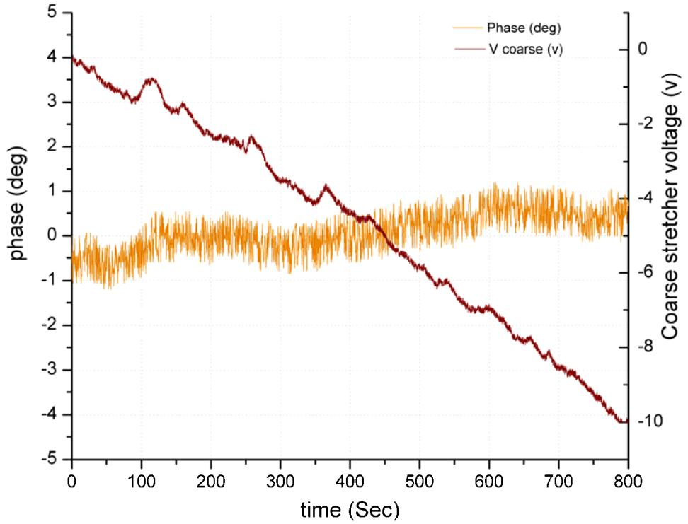
**Figure 28:** Test of the phase incurred on 5 km of fiber at 20 GHz with the correction system on (from 0 sec to 800 sec) with an OA located just before the far-end photomixer (refer to figure 12). No movement of the fiber has been applied.
