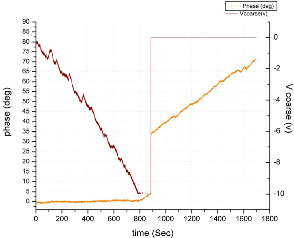
**Figure 27:** Test of the phase incurred on 5 km of fiber at 20 GHz with the correction system on (from 0 sec to 800 sec) and off from (800 sec to 1700 sec) with an OA located just before the far-end photomixer (refer to figure 12). No movement of the fiber has been applied.
