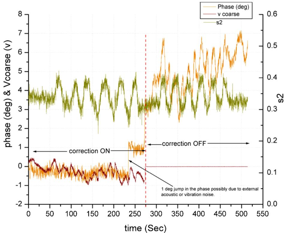
**Figure 24:** 10 km correction is on and undergoes cyclical bending from 0 to 275 sec., then the correction is turned off from 275 sec to 525sec. The bend radius was changing from 2.5 inch to 26 inches.
