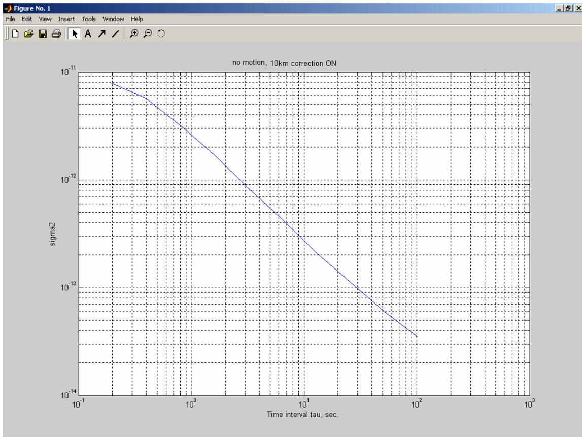
**Figure 20:** the measurement of the Allan variance of the phase in figure 19(10 km, for a reference frequency of 20 GHz and sampling time of 0.2 sec.
