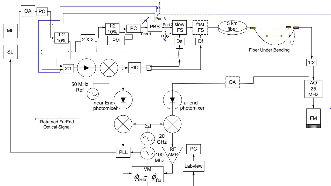
**Figure 12 - Faraday Mirror** test setup for the line length correction system without the use of an optical circulator. Instead we used the combination of PBS and faraday mirror to rout the light signal back to the near end as shown in the blue line
