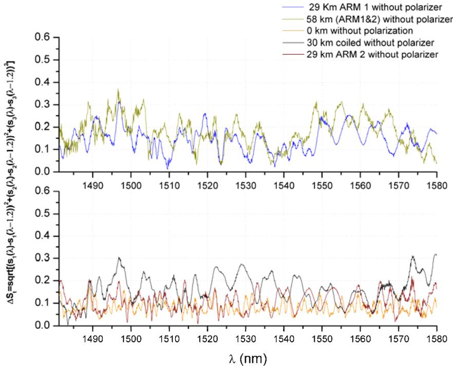
**Figure 10** : The 1.2nm-variation in  $S_T$  (as described by Eq3). The  $S_T$  parameter is normalized to the output SOP of the wavelength that is 1.2 nm preceding it
