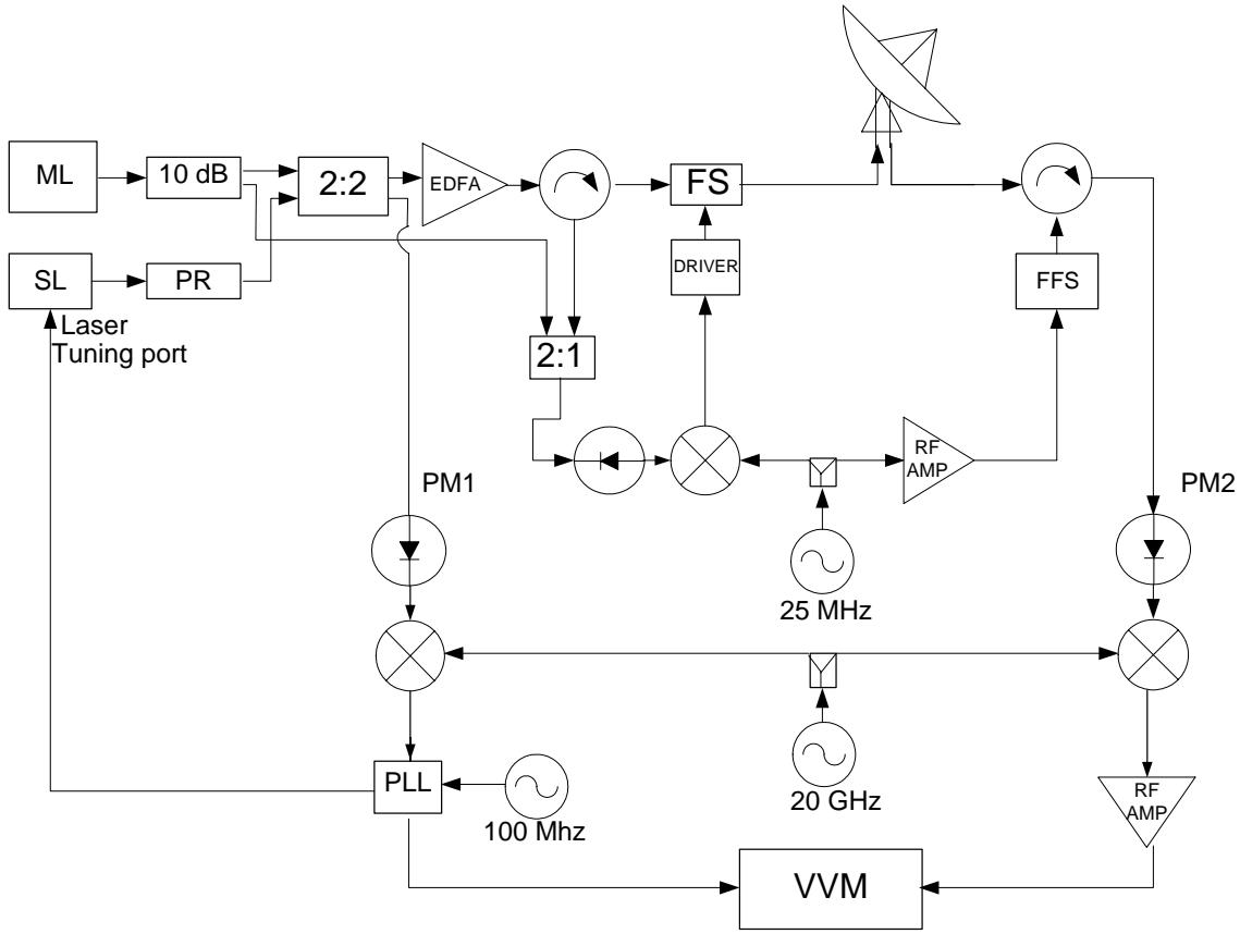
**Figure 1:** Line length correction previous test setup – Note that the antenna cable wraps are traversed twice.
