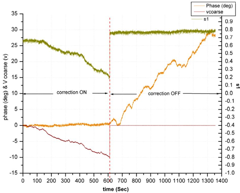
**Figure 18:** Test of the phase incurred on 10 km of fiber at 20 GHz with the correction system on and off (no movement of the fiber).
