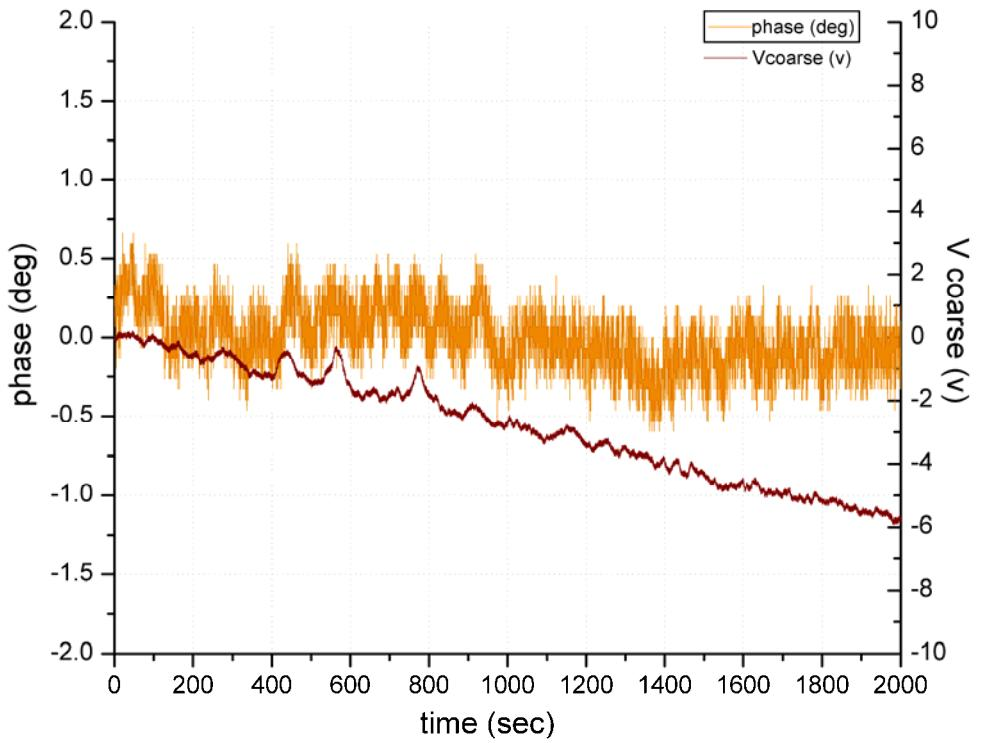
**Figure 16:** Test of the phase incurred on 5 km of fiber at 20 GHz with the correction system on and no movement of the fiber.
