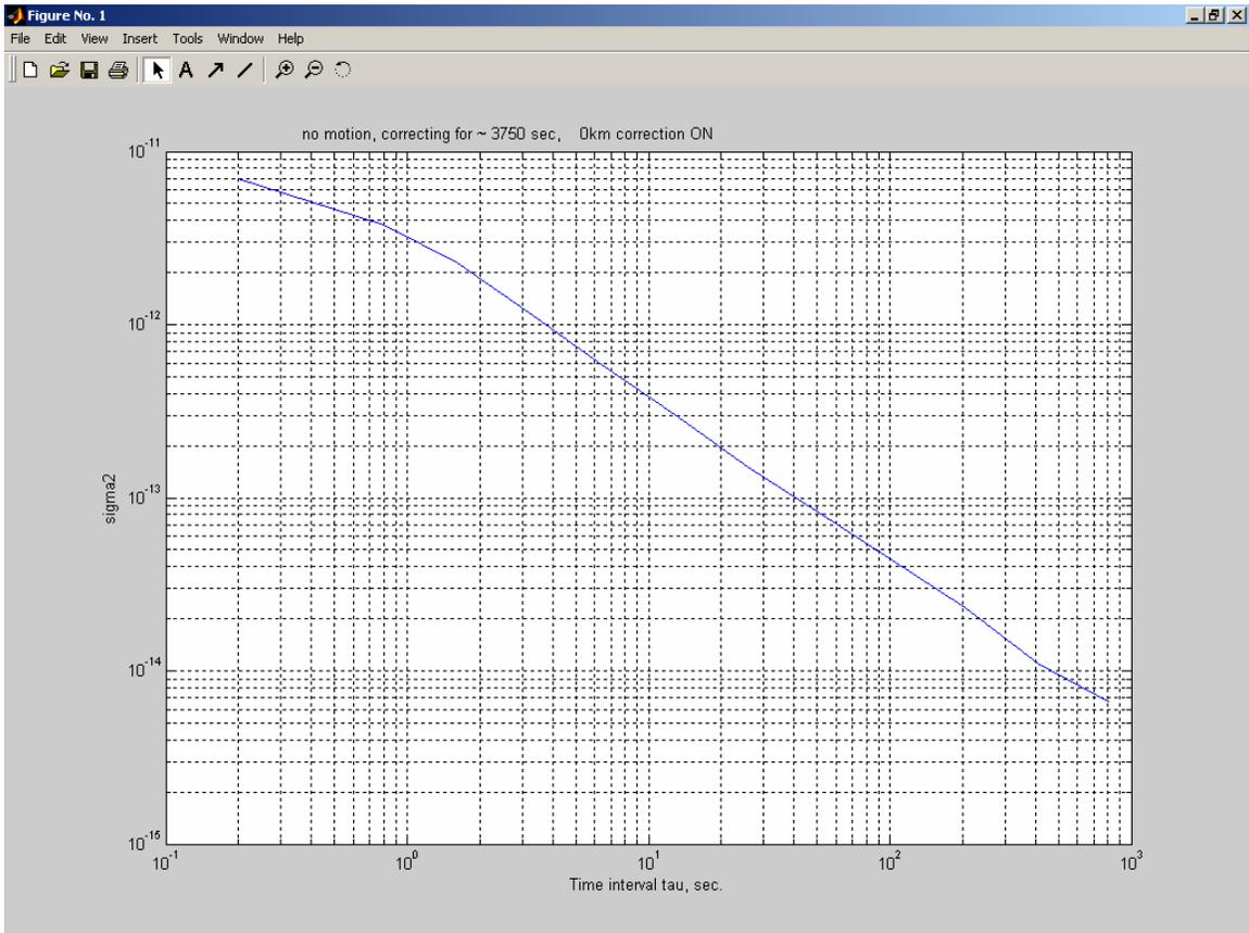
**Figure 14:** The measurement of the Allan variance of the phase in figure 13 (1m fiber length), for a reference frequency of 20 GHz and sampling time of 0.2 sec.
