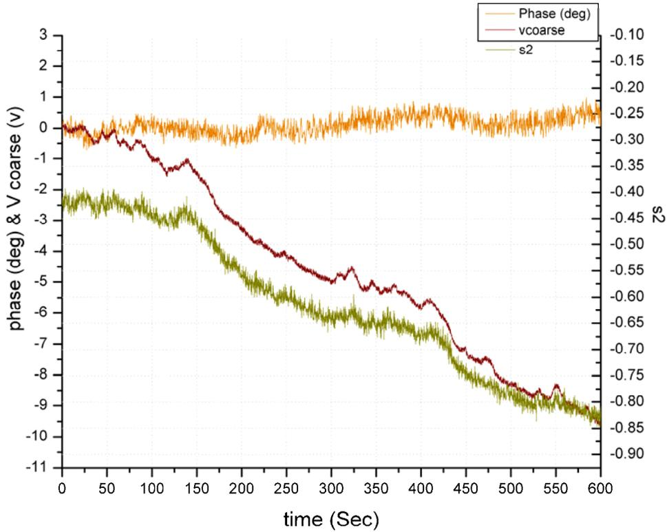
**Figure 19:** Test of the phase incurred on 10 km of fiber at 20 GHz (no movement of the fiber). This is a zoomed section of the previous plot.
