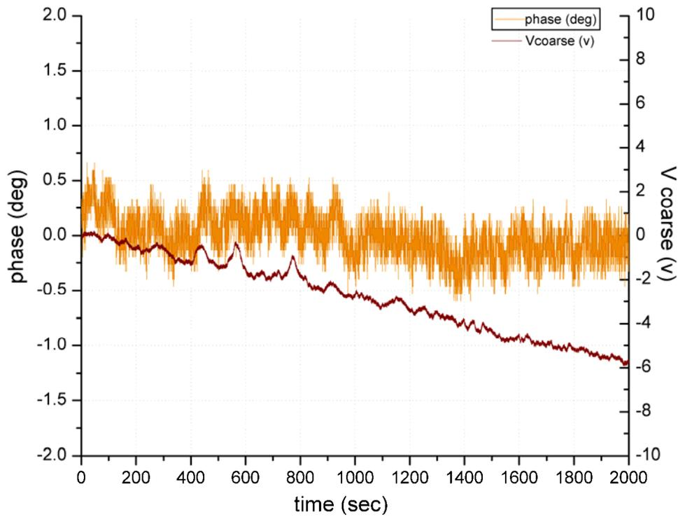
**Figure 16:** Test of the phase incurred on 5 km of fiber at 20 GHz with the correction system on and no movement of the fiber.
