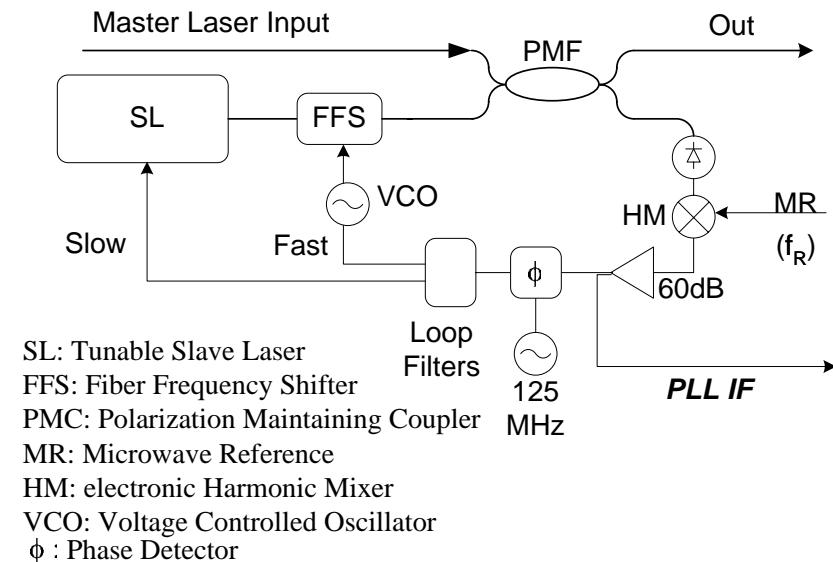
**Figure 29** Schematic of the laser synthesizer.
