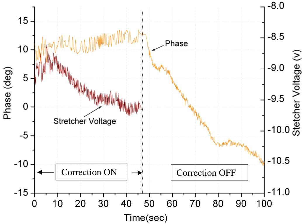
**Figure 32 108GHz locked beatnote phase measurement over 10km while correcting for 47 sec and un-correcting for 53 sec.**
