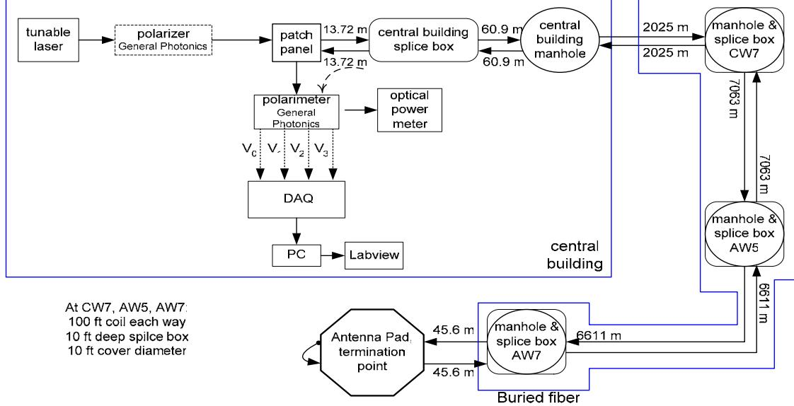
**Figure 8:** Test setup for measuring the variation of the polarization of the laser light traveling through the buried fiber cable of the EVLA site while scanning the wavelength of a tunable laser source
