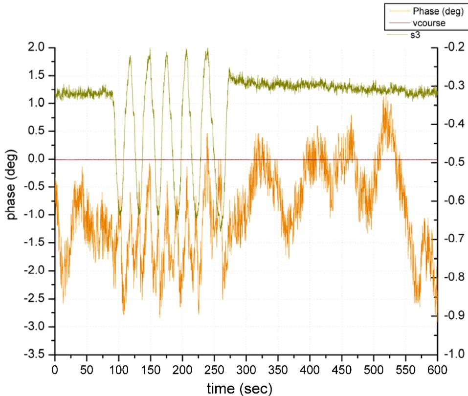
**Figure 21:** 5 km correction is **OFF** all the time. From 100 to 275 sec the fiber was bent and unbent multiple times, the bend radius was changing from 2.5 inch to 26 inch. From 275 to 600 sec, the bending is stopped.
