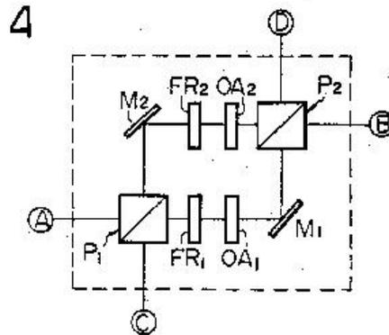
**Figure 5** - US Patent #4,650,289 “Optical Circulator – Polarization Independent Input Type” Mar 17, 1987
