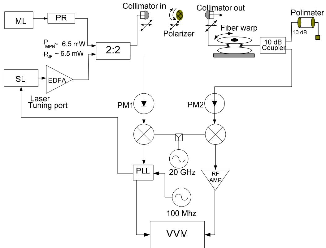
**Figure 6** - Test setup for measurement of phase fluctuation due to fiber movement, using two lightwaves with polarization alignment enforced by use of a free-space polarizer. There are no circulators in the receiving system.
