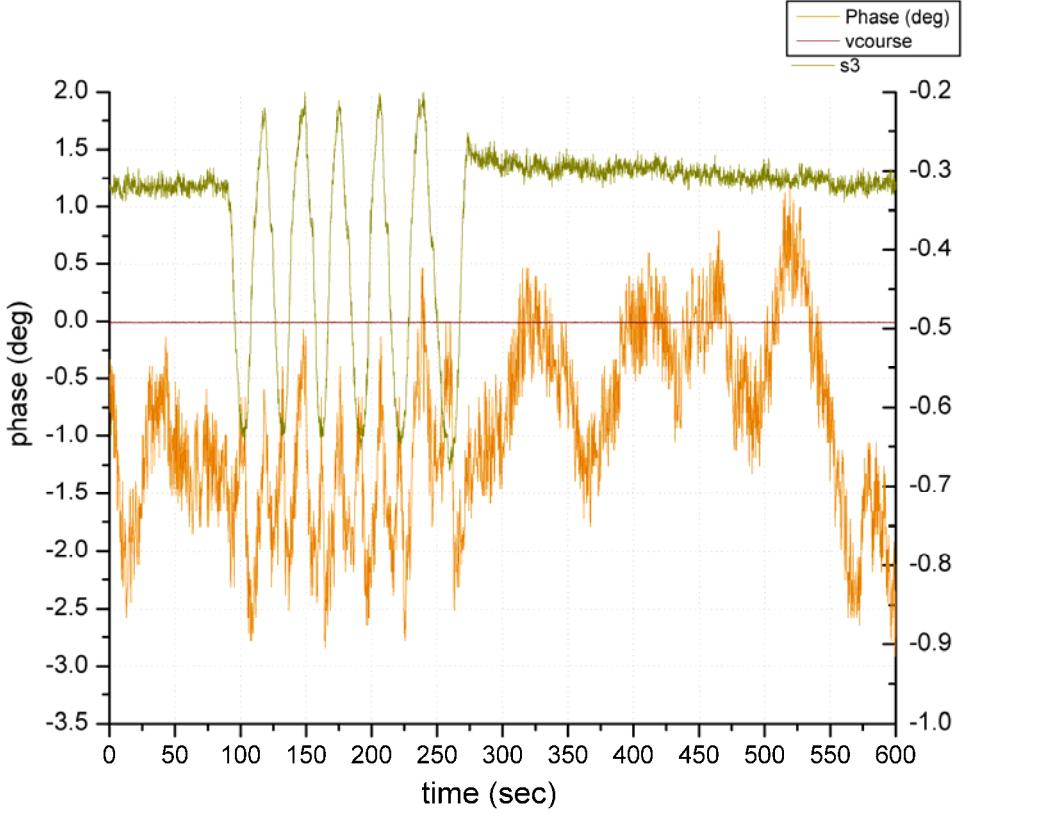
**Figure 21:** 5 km correction is **OFF** all the time. From 100 to 275 sec the fiber was bent and unbent multiple times, the bend radius was changing from 2.5 inch to 26 inch. From 275 to 600 sec, the bending is stopped.
