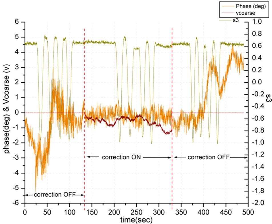
**Figure 25:** 5 Km with twisting ½ inch of fiber from 0 to + 360 deg and then back from +360 to 0 deg . The correction is OFF from 0 to 130 sec, then the correction is ON from 125 sec to 327sec, and finally correction is OFF from 327sec to 490 sec.
