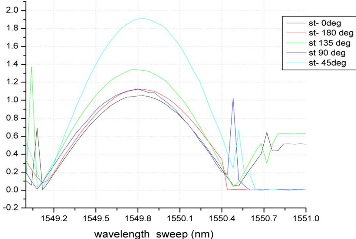
**Figure 4:** Test Result of State-of-Polarization-Dispersion of Optical Circulator. The vertical axis is  $S_T$  (see Eq(1) above). Each trace corresponds to a specific input polarization angle as shown in the key. Peaks and jumps occurring outside the 1549.1–1550.4 range are artifacts of the data acquisition and should be ignored.
