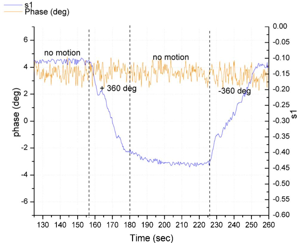
**Figure 11** - Results of test setup Figure #6 (with the polarizer is removed & the Master and slave are misaligned by  $S_T = 0.2$ ) .The phase fluctuation resulted by moving the fiber by +360 azimuth rotation and back by -360
