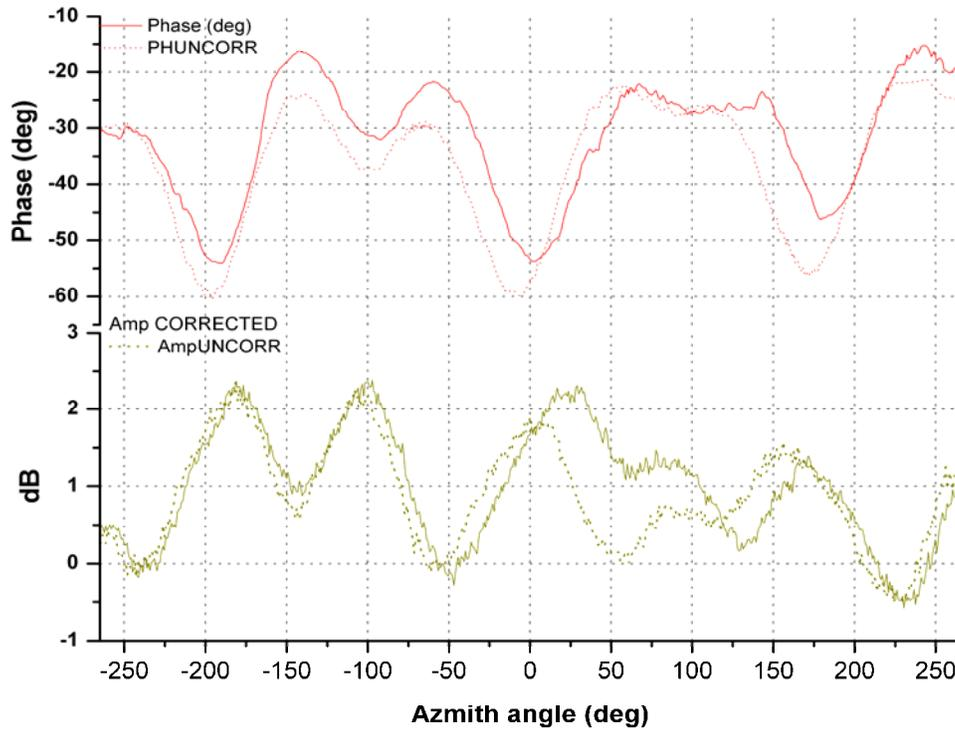
**Figure 2** - Phase fluctuation of the 20 GHz beatnote versus azimuth position (red trace-top). The solid line is with the line length correction ON and the dashed line is with the correction OFF. The phase artifact is not affected by the correction, and has some correlation with the variation of the beatnote amplitude (bottom trace).
