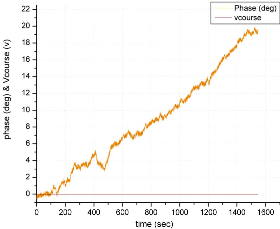
**Figure 15:** Test of the phase incurred on 5 km of fiber at 20 GHz with the correction system off and no movement of the fiber.
