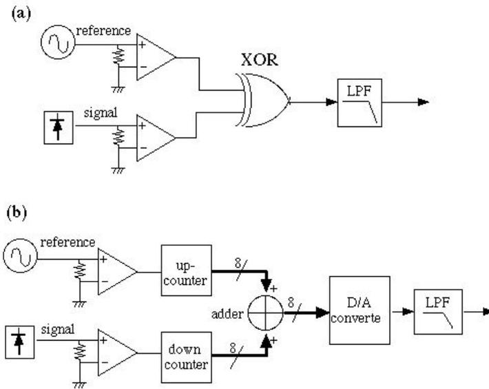
**Figure.1:** Schematic diagram of (a) conventional digital PSD and (b) digital phase and frequency discriminator (DPFD)
