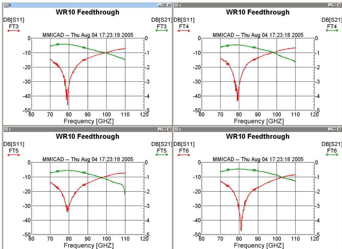
Fig. 7. Measurements on four feedthrough assemblies with epoxy windows.  $|S_{11}|$  (red, dB, left scale),  $|S_{21}|$  (green, dB, right scale).
