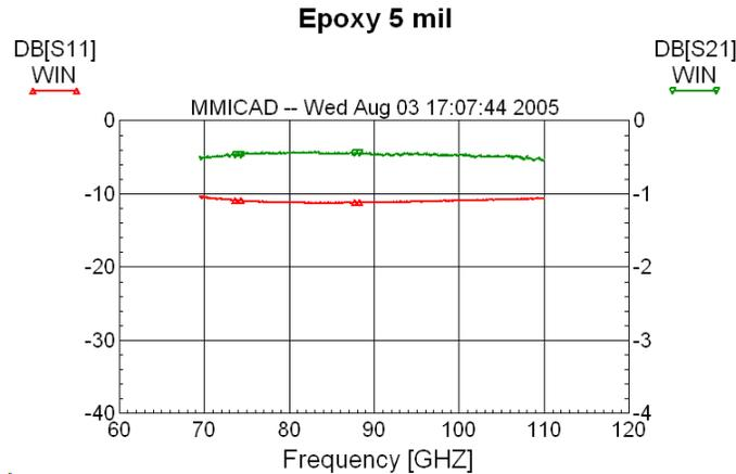
Fig. 4.  $|S_{11}|$  (red, dB, left scale) and  $|S_{21}|$  (green, dB, right scale) of a 5-mil section of WR-10 filled with Epo-Tek 301-2.
