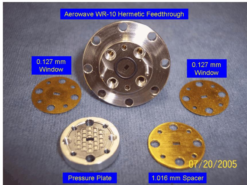
**Fig. 10. Components of the feedthrough.**
