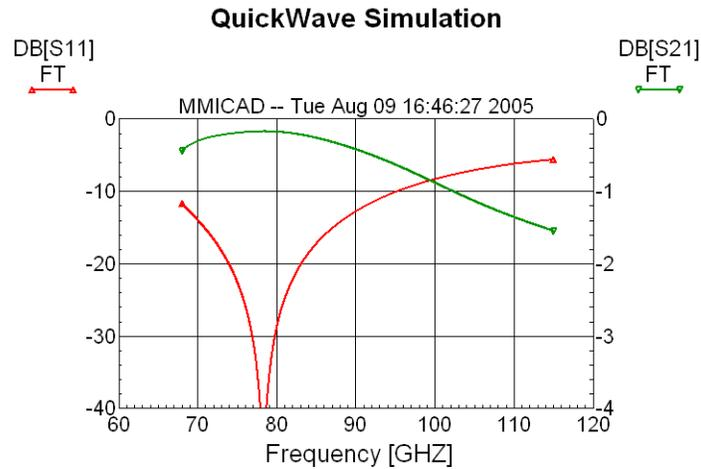
Fig. 6. QuickWave Simulation of the feedthrough assembly in Fig. 1.  $|S_{11}|$  (red, dB, left scale) and  $|S_{21}|$  (green, dB, right scale).
