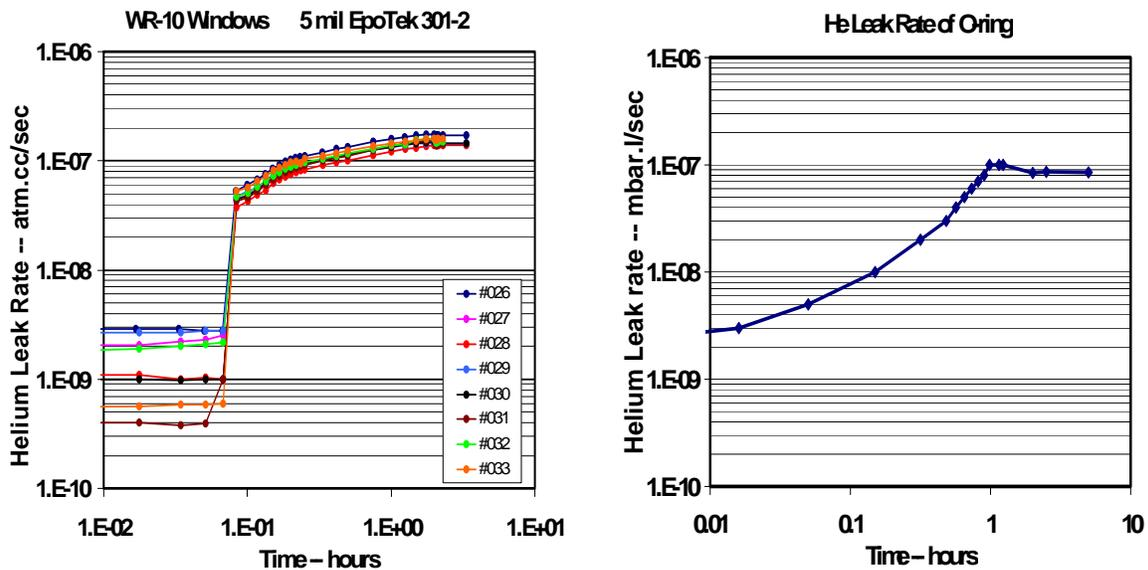
Fig. 5. Left: Helium leak rate as a function of time, for eight windows. Right: Leak rate of the O-ring. The window under test was covered with a balloon full of helium during the measurements.
