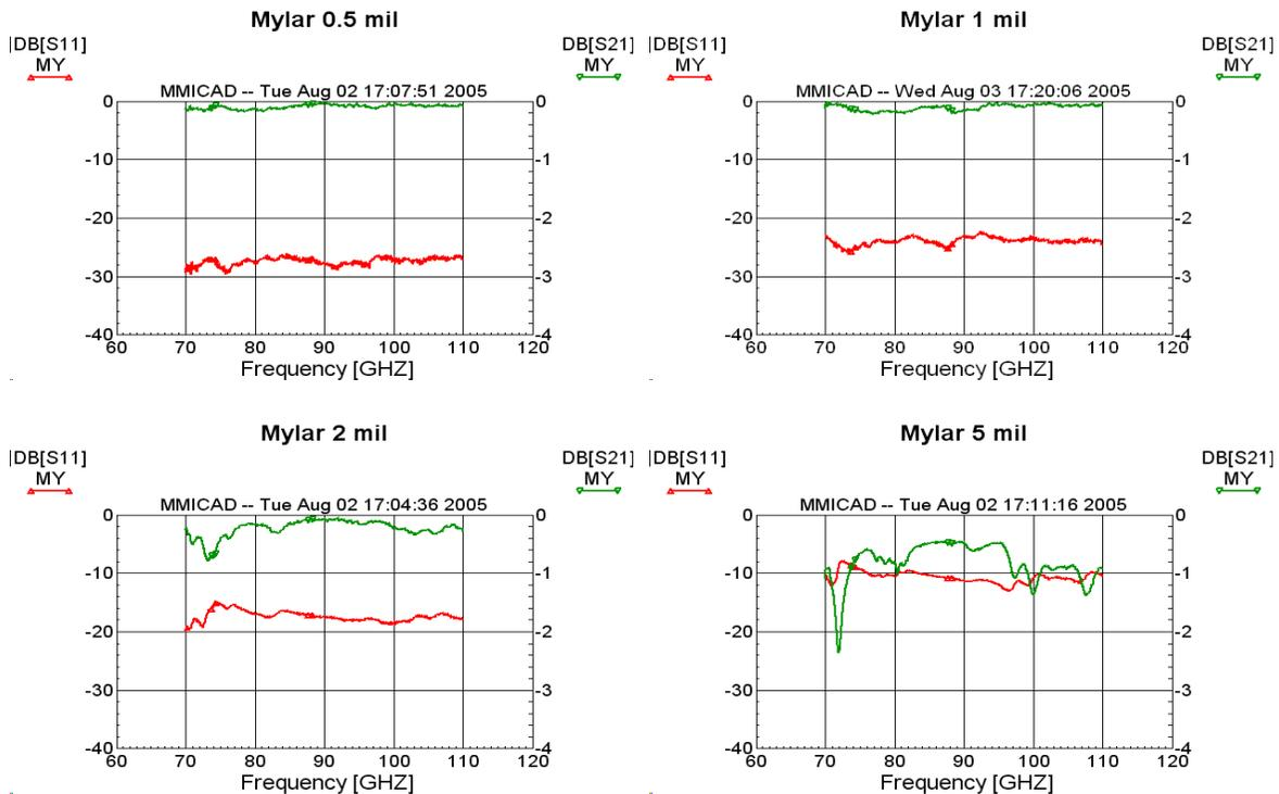
Fig. 3.  $|S_{11}|$  (red, dB, left scale) and  $|S_{21}|$  (green, dB, right scale) of Mylar sheets of several thicknesses clamped between the WR-10 waveguide flanges of an Agilent 8510 VNA.
