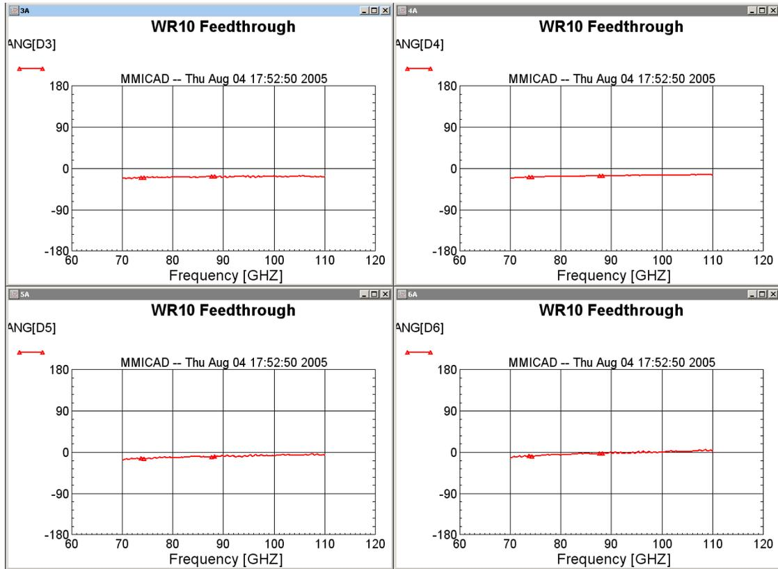
**Fig. 8. Measured phase of  $S_{21}$  for the same four feedthroughs measured in Fig. 7. The phase is relative to that of a 0.740" length of waveguide.**
