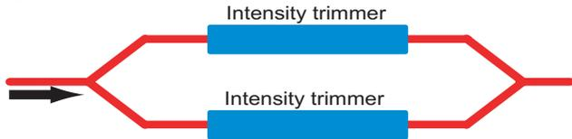
Fig. 2 MZ modulator with intensity trimmers.
