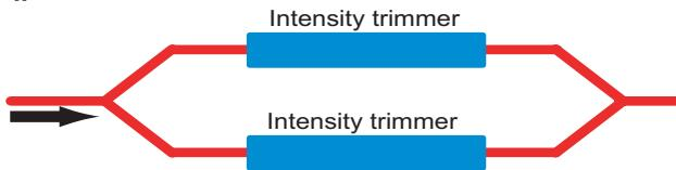
*Fig. 2 MZ modulator with intensity trimmers.*
