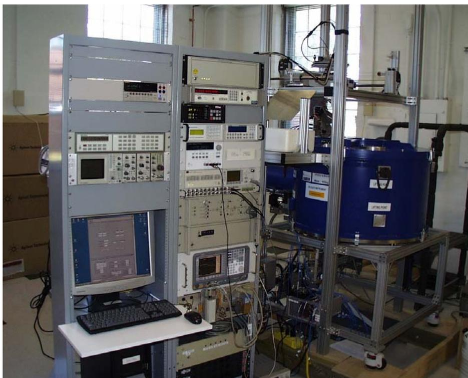
Figure 1. Cryostat in test frame with electronics racks.
