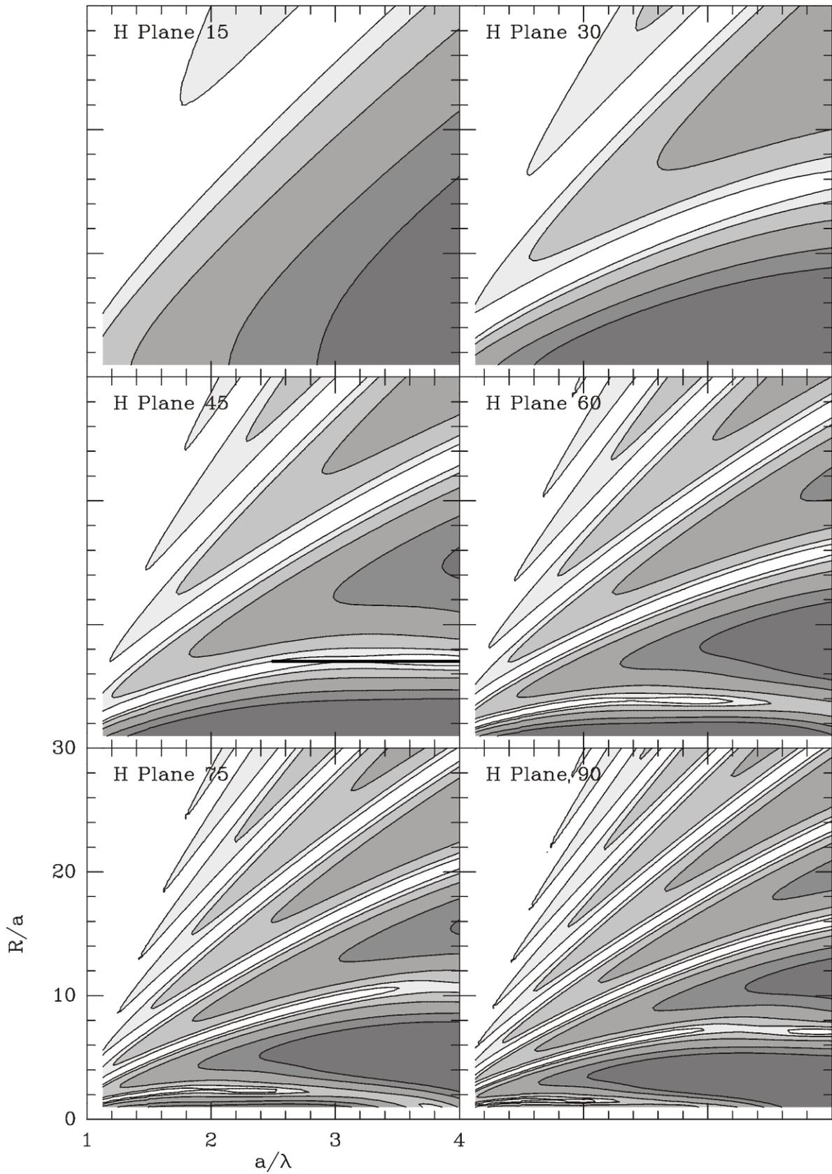
**Figure 1: Results for H-plane bends, versus  $a/\lambda$  and  $R/a$  for discrete values of angles in 15 degrees increments. The contour values represent the fractional power lost in the 3 first spurious modes. The contour values are 0.01 (-20dB), 0.03 (-15dB), 0.1 (-10dB), 0.3 (-5dB), and 0.5 (-3dB). The horizontal line overlaid on the 45° box points to a "quiet zone"; see text for comments.**
