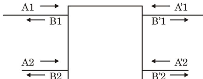
**Figure 5: Four-port schematic of mode conversion in the bend. The index 1 belongs to the fundamental mode, and index 2 to the dominant trapped overmode.**
