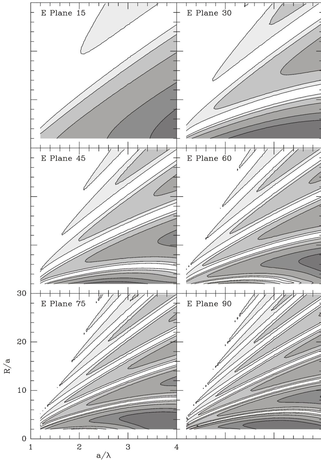
**Figure 2: Results for E-plane bends, versus  $a/\lambda$  and  $R/a$  for discrete values of angles in 15 degrees increments. The contour values represent the fractional power lost in the 6 first spurious modes. The contour values are 0.01 (-20dB), 0.03 (-15dB), 0.1 (-10dB), 0.3 (-5dB), and 0.5 (-3dB).**
