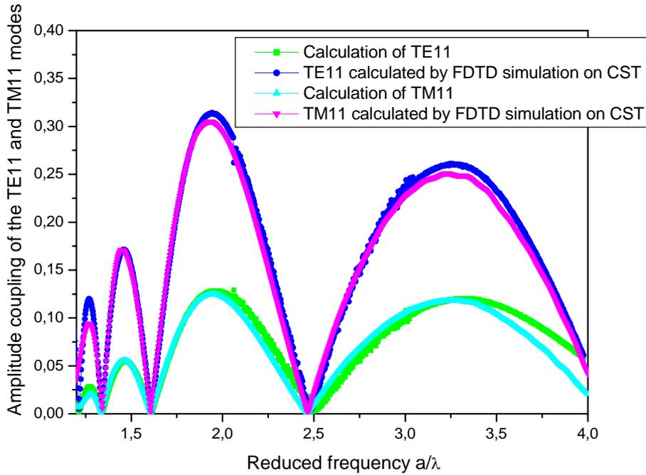
**Figure 4: Comparison of FDTD simulation of TE<sub>11</sub> and TM<sub>11</sub> amplitudes coupling with analytical calculations for six spurious modes**
