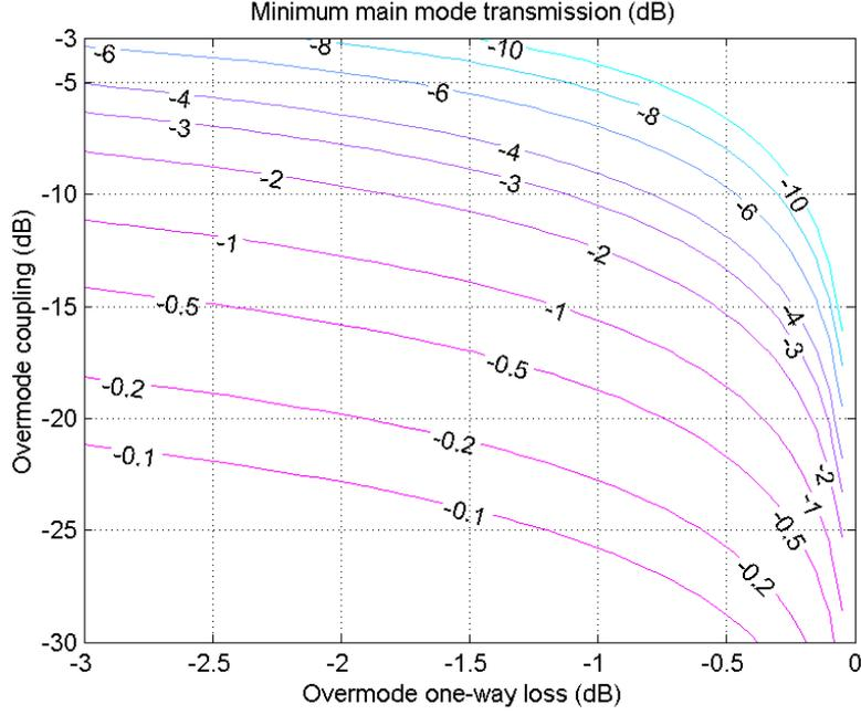
Figure 6. Minimum transmission contours (dB), versus the one-way (one half round trip) loss of the overmode, expressed in dB ( $20 \log(\rho)$ ) and the coupling between the fundamental and the overmode, also expressed in dB ( $20 \log(p)$ ).
