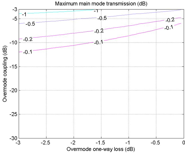
Figure 7. Maximum transmission, same units as in Figure 6. The loss at maximum transmission is generally small enough that, for practical purposes, it is not necessary to distinguish between the minimum transmission and the amplitude of the resonant dip.
