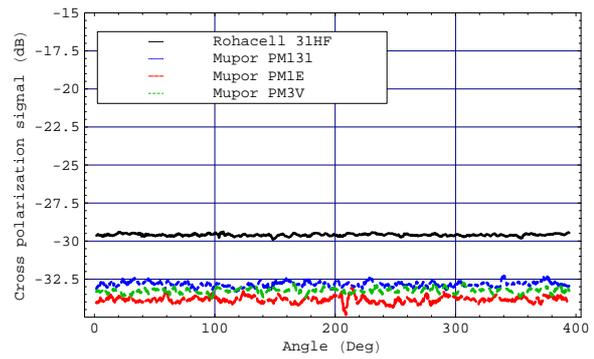
(b) Mupor® PM131, Mupor® M1E, Mupor® M3V, Rohacell® 31 HF measured at 648 GHz
