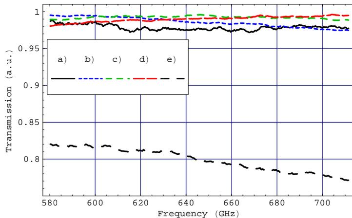
Fig. 6: Transmission of different materials: a) GORE-TEX<sup>®</sup> RA 7956, b) Mupor<sup>®</sup> PM131, c) Mupor<sup>®</sup> M1E, d) Mupor<sup>®</sup> M3V, e) Rohacell<sup>®</sup> 31 HF
