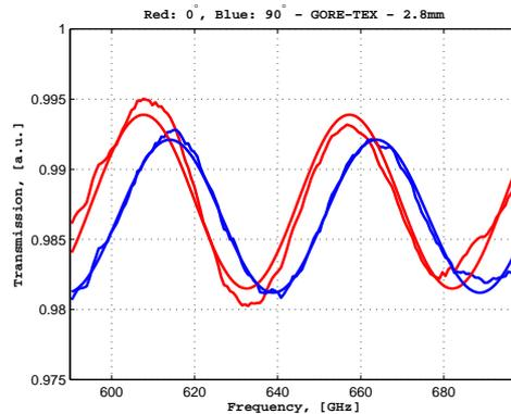
Fig. 2: Transmission for a 2.8 mm GORE-TEX<sup>®</sup> GR slab at band 9 frequencies.
