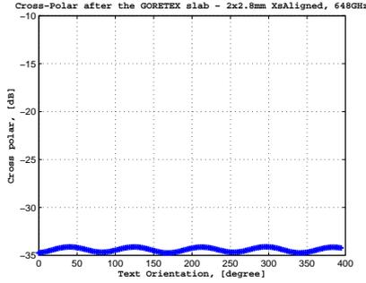
Fig. 5: Cross-polarization introduced by a pair of same thickness sheet samples (GORE-TEX<sup>®</sup> GR 2.8 mm) facing each other at 90°.  $f = 648 \text{ GHz}$ .
