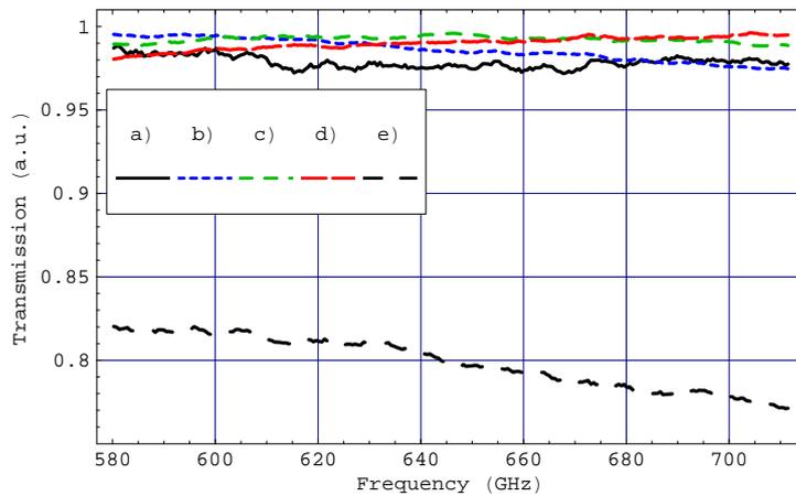
Fig. 6: Transmission of different materials: a) GORE-TEX<sup>®</sup> RA 7956, b) Mupor<sup>®</sup> PM131, c) Mupor<sup>®</sup> M1E, d) Mupor<sup>®</sup> M3V, e) Rohacell<sup>®</sup> 31 HF
