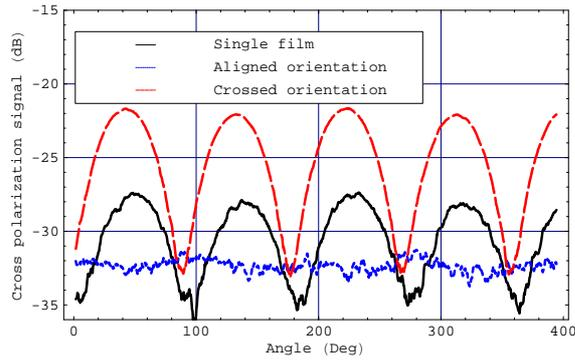
(a) GORE-TEX® RA 7956 at 702 GHz. Single film and a sandwich of crossed and co-aligned films are shown.
