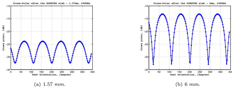
Fig. 4: Cross-polarization introduced by 1.57 mm and 6 mm slabs of GORE-TEX<sup>®</sup> GR at 648 GHz.
