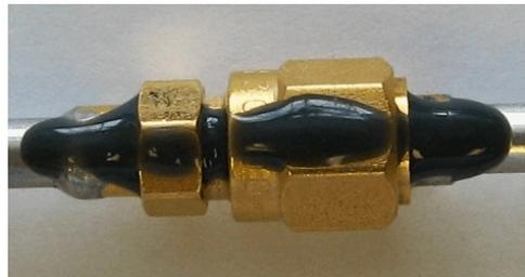
Applying an adhesive to the threads of an SMA connector, as opposed to striping, is considered undesirable for the following reasons: (i) During connector engagement, the adhesive can be
