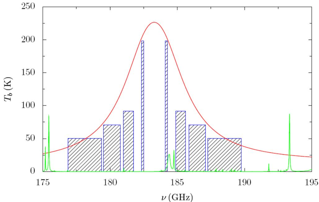
Figure 1. RF coverage produced by the filters in the prototype radiometers.
