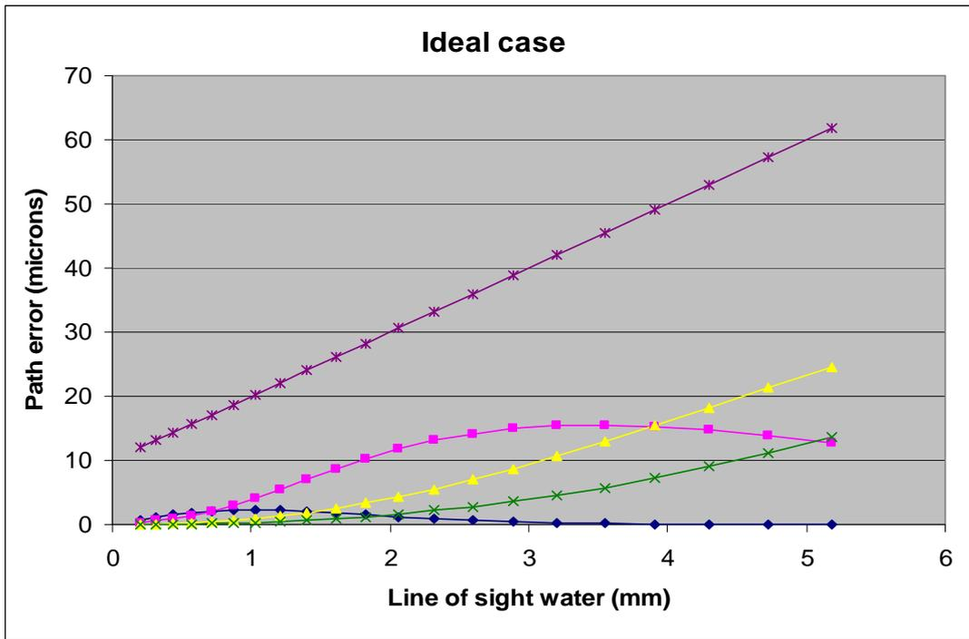
Figure 12. Effect of 0.1% change in each centre frequency on estimated path – clear sky case.
