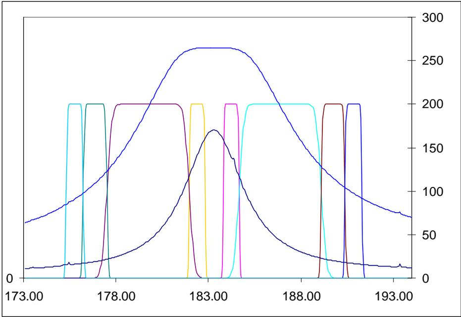
Figure 7. Filters optimized for “cloud” case – i.e. discriminates against continuum.
