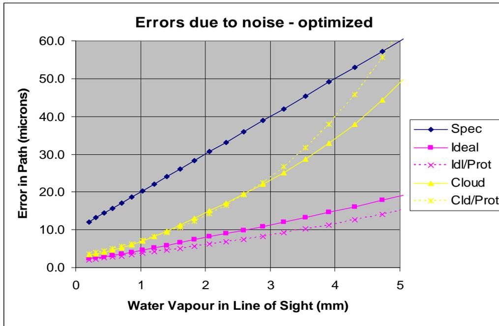
Figure 10. Production radiometer performance with equivalent for prototype for comparison. Here, for interest, I have plotted as dotted curves the sensitivities of the prototype radiometers, assuming the same parameters for noise temperature, loss and so on, but allowing for the
