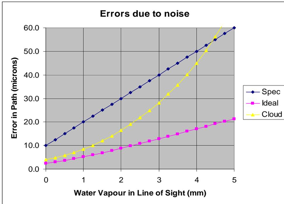
Figure 5. Estimated errors in path using filters in Table 2 and Figure 2.
