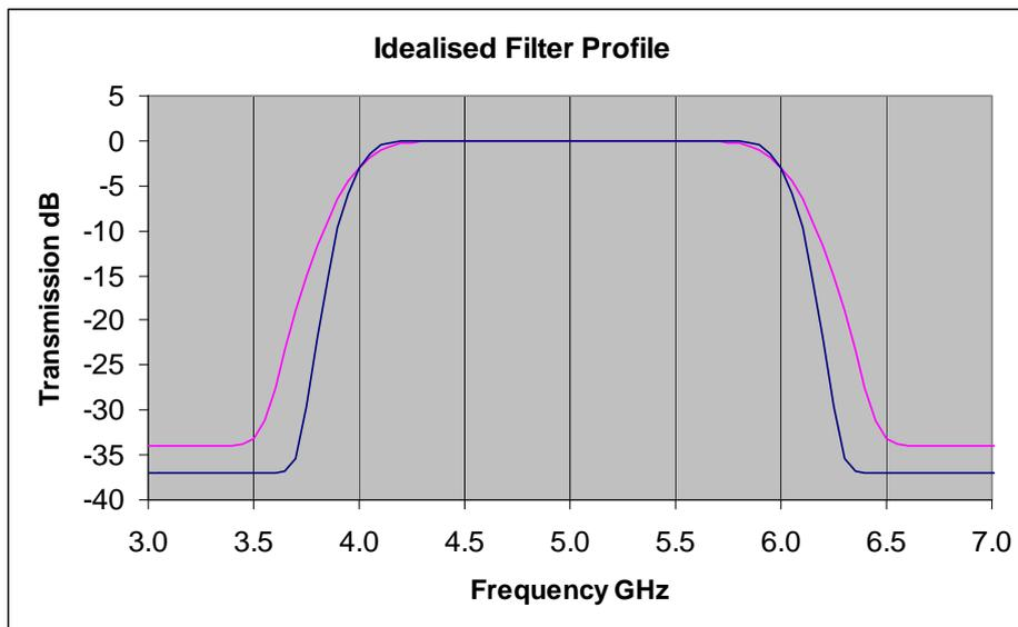
Figure 3. Illustrating the form of filter profile use in the model.
