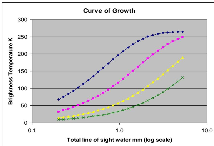
Figure 4. Growth of Brightness Temperature with line of sight water for filters in Table 2.
