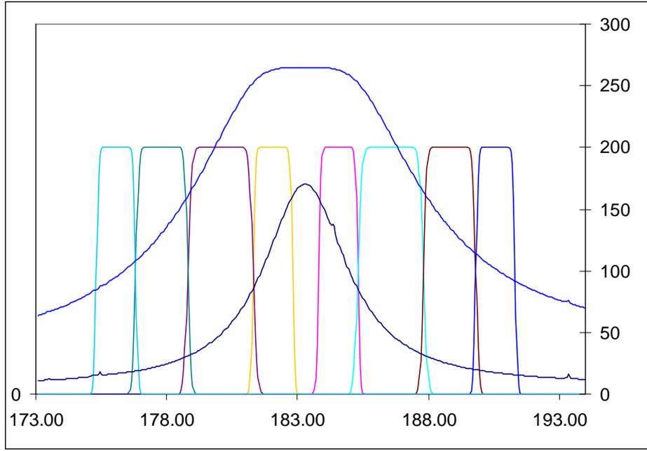
Figure 9. RF frequency coverage for filters in Table 4 together with the line emission profile for 0.5 and 4mm of water vapour.
