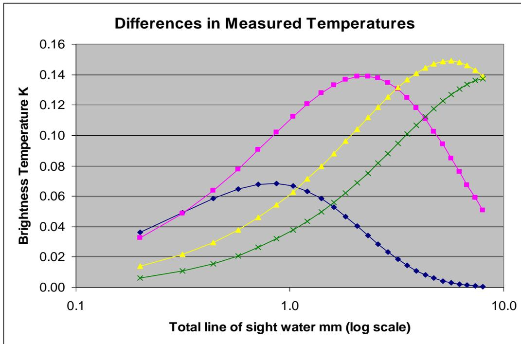
Figure 11. Effect of 0.1% change in the centre frequencies of the IF filters.
