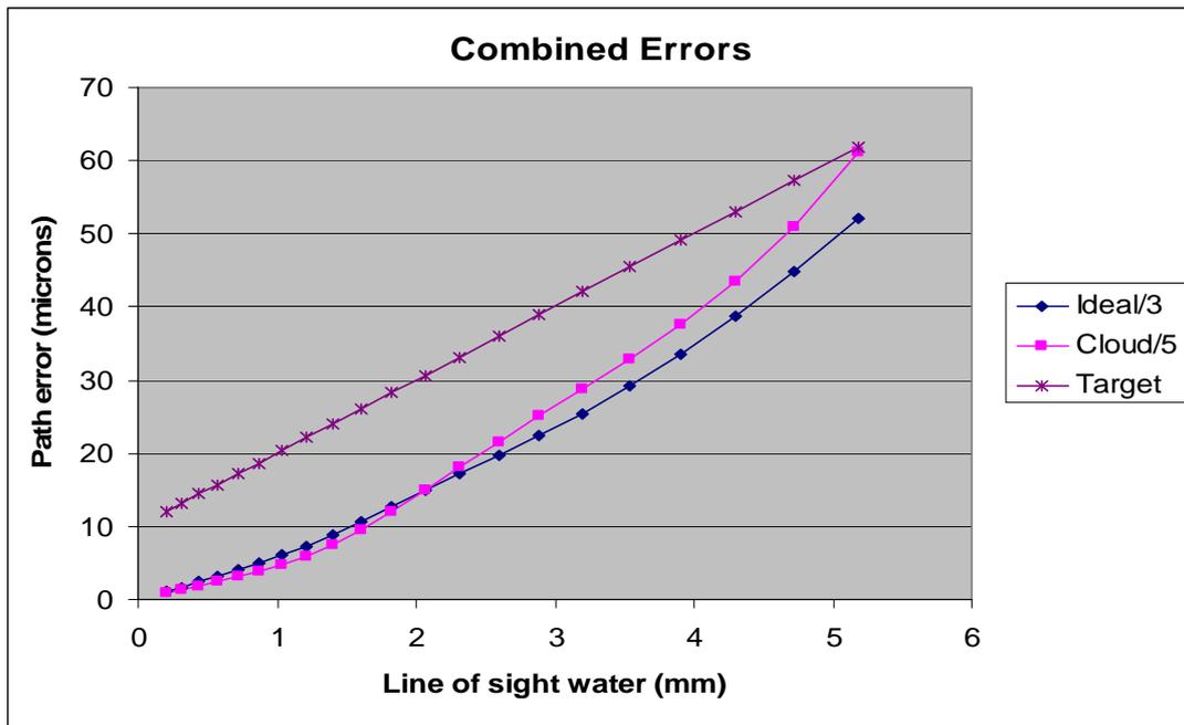
Figure 15. Results of combination of filter and sideband errors (divided by factors of 3 and 5).
