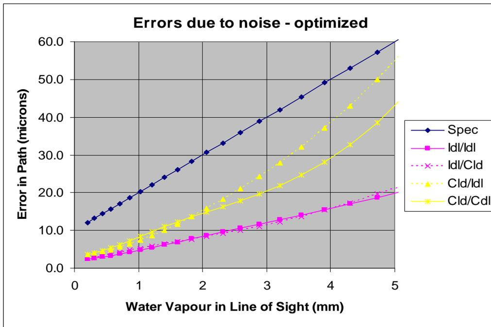
Figure 8. Estimated errors in path for the two sets of filters specified by Table 3.
