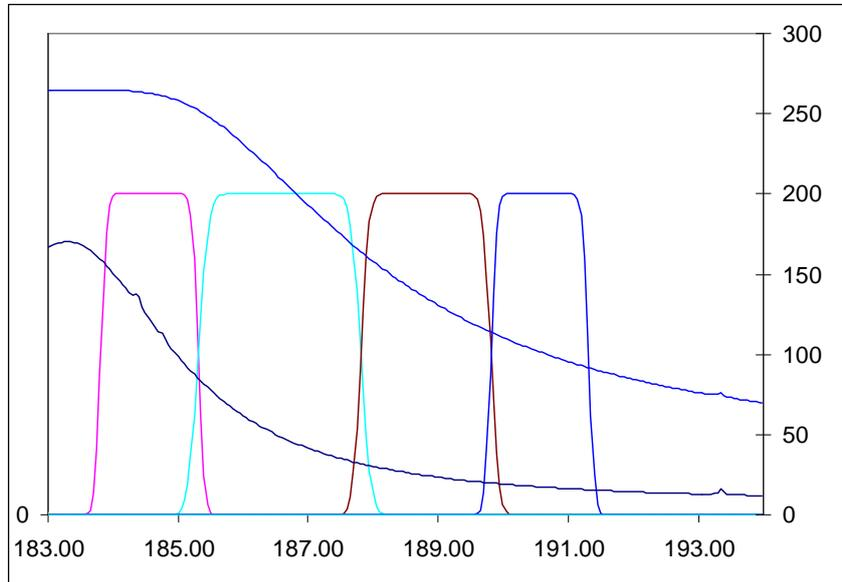
Figure 16. Filters with edge widths equal to bandwidth divided by 20.
