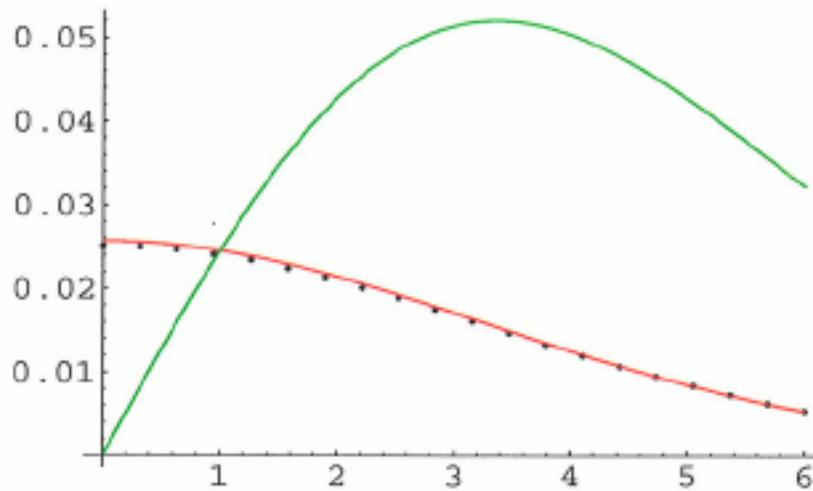
Figure 5. The convolution between the projected cone area and the BSDF function (red line) and the area weighted convolution (green line) for 500 nm wavelength.
