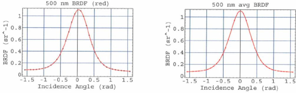
Figure 1. (a) Measured BRDF function in the meridian plane and (b) the average BRDF value for the perpendicular plane
