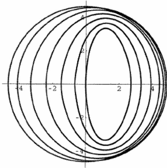
Figure 4. The projected cone views of the subreflector from the different positions on the primary reflector.
