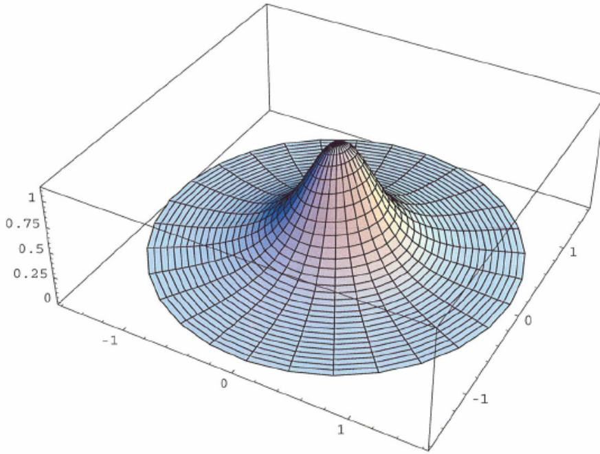
Figure 2. Assumed 2-D form of the BSDF function of the primary panels.
