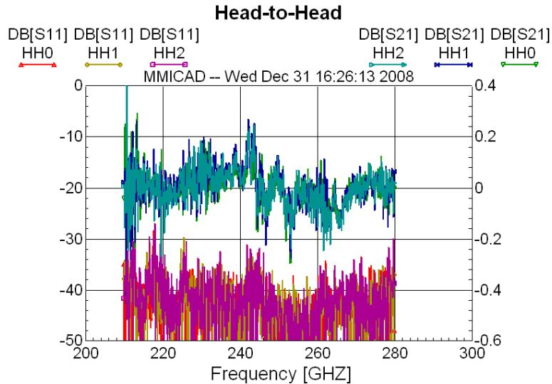
Fig. 6. Measurements with the VNA heads connected directly together, before, during, and after the loss measurements.
