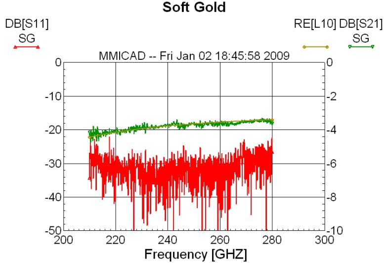
Fig. 3. Soft gold plated waveguide. The best-fit loss curve is obtained for  $\sigma = 3.84 \times 10^7$  S/m.
