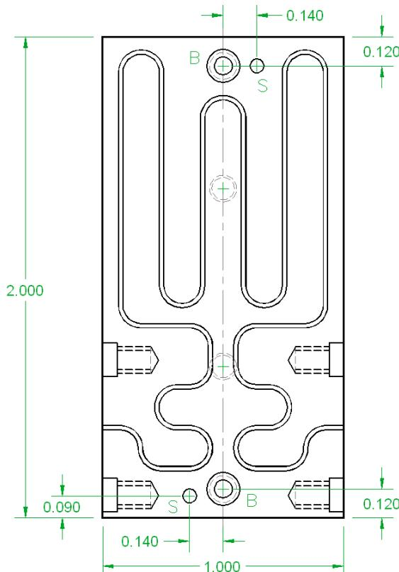
Fig. 1. The waveguide pattern in the test pieces. The waveguide is WR-3.7 (0.037" x 0.0185"). The total waveguide length is 10.000 inches.
