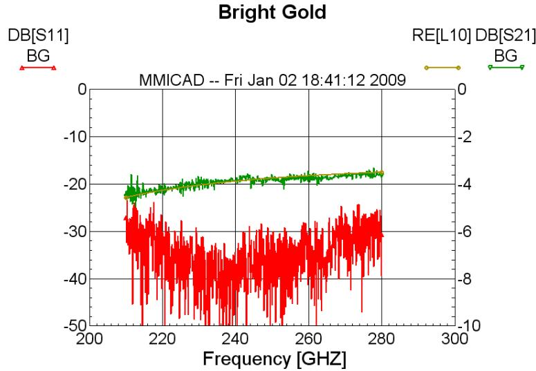
Fig. 2. Bright-gold plated waveguide. The best-fit loss curve is obtained for  $\sigma = 3.63 \times 10^7$  S/m.
