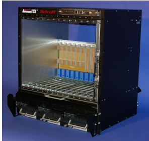
(a) An enclosure with copper mesh interconnect provided by an ATCA standard backplane. This backplane supports 40 Gb/s all-to-all connections for up to 14 cards.
