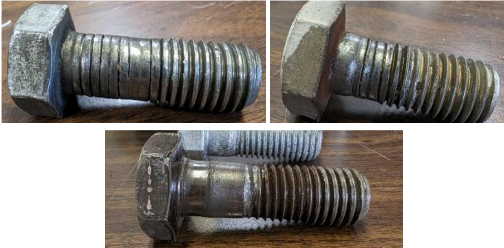
Figure 12: Left – SAE grade 5 bolt 1 (10d). Right – A325 bolt 1 (7d). Bottom – A325 bolt 4 (9d).
