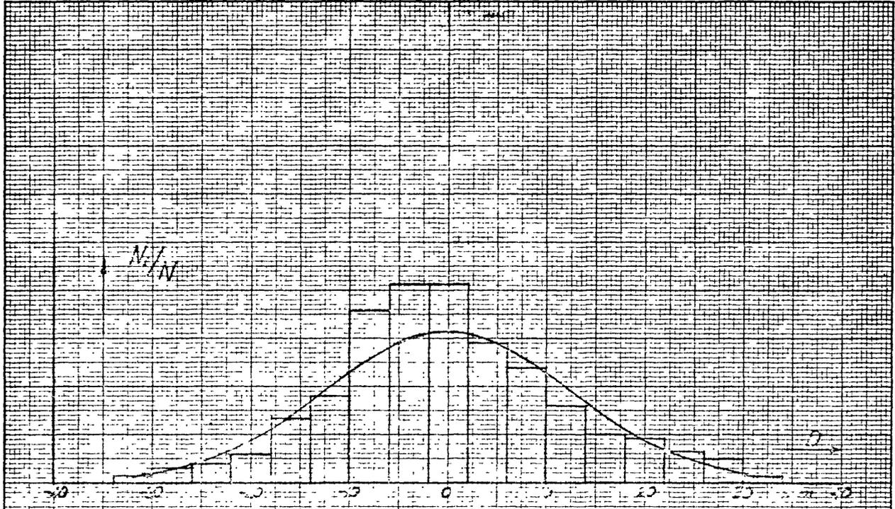
Fig. 10a. The distribution of the measured deviations of the 00-15m antenna from the best-fitting paraboloid ( $N = 293$ ,  $\bar{x} = 51.7340$ ).
