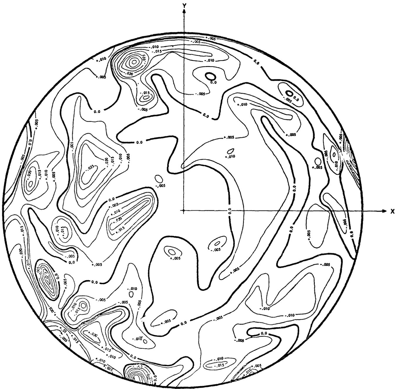
Figure 10. Contour map representation of the surface deviations of the 85-foot reflector from best fitting paraboloid measured in zenith position. Distances are measured in a direction normal to the reflector surface, positive direction towards the focal point. Interval = .005 ft., 1.5 mm.
