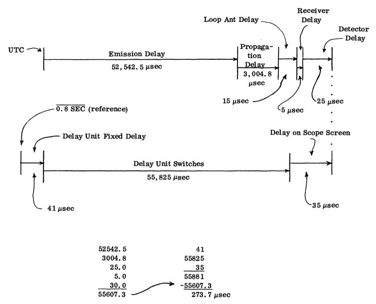
The  $\overline{0.8 \text{ SEC}}$  reference signal from the VLB CONTROL is 273.7 ± 25 µsec earlier than UTC.
