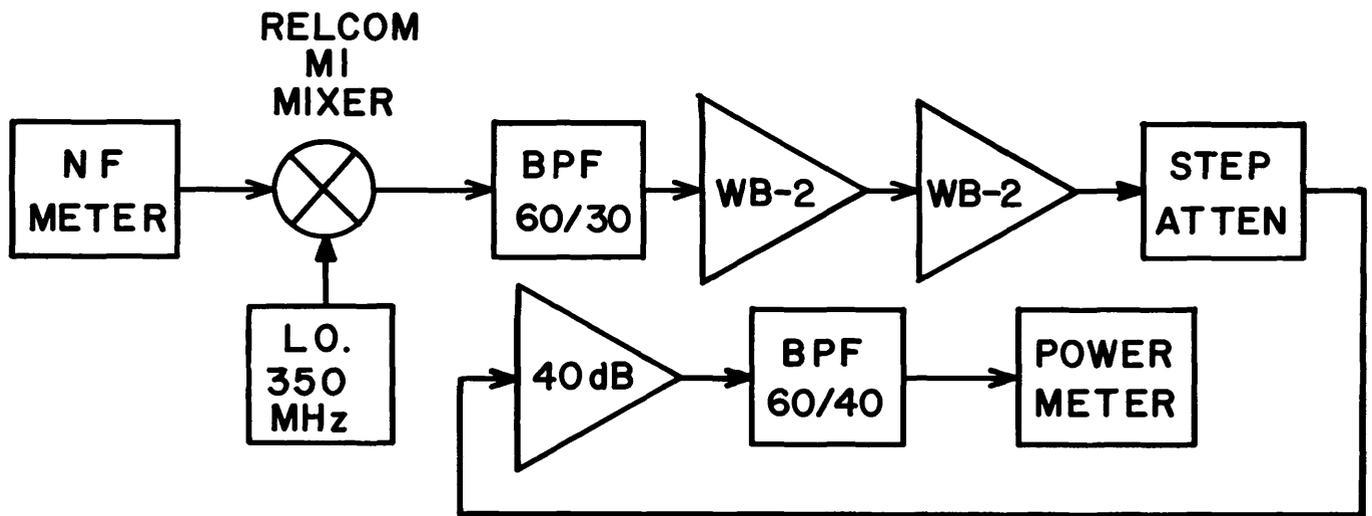
NOISE FIGURE WITH ABOVE SET UP = 8.0 dB
