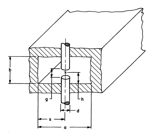
Figure 1: MOUNTING POST GEOMETRY.
