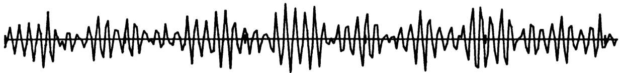
FIGURE 12. INTERFERENCE PATTERN BETWEEN INCOMING AND TRANSMITTED WAVES WITH VARYING FREQUENCY (BOTTOM) AND ITS FOURIER TRANSFORM (TOP) WHICH SHOWS THE RETURN LOSS (REFLECTION COEFFICIENT) AS A FUNCTION OF DISTANCE FROM THE REFLECTOMETER. THIS SPECTRUM WAS TAKEN ON THE 140-FOOT BEFORE ANY MODIFICATIONS WERE MADE TO SUPPRESS REFLECTIONS. REFLECTIONS ARE FROM (A AND B) THE TOP OF THE CASSEGRAIN HOUSE, (C) THE CASSEGRAIN FEEDS, AND (D) THE INNER DISH SURFACE.
