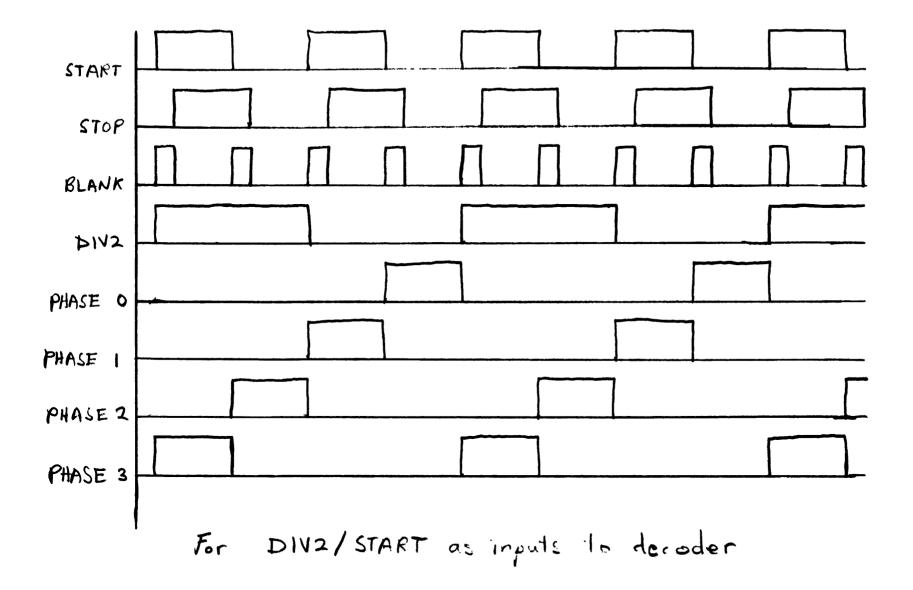
Figure 6. Signals from logic circuitry.
