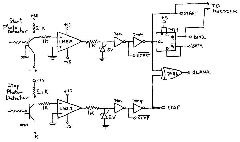
Figure 4. Photodetection and logic circuitry.
