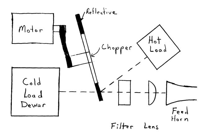
Figure 7. Possible set-up with hot load in furnace.
