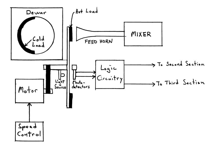
Figure 2. First section with mixer being tested.
