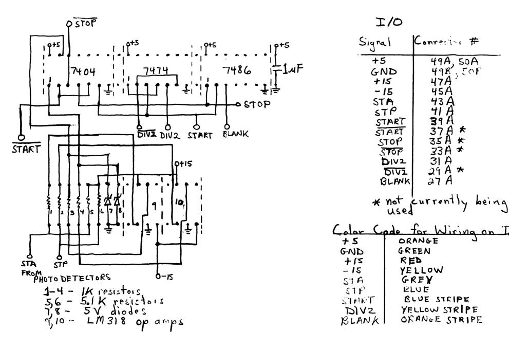
Figure 5. Wiring and input/output of logic circuit board.
