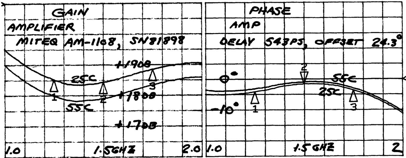
Fig. 1. Test results for L-band filter and amplifier.
