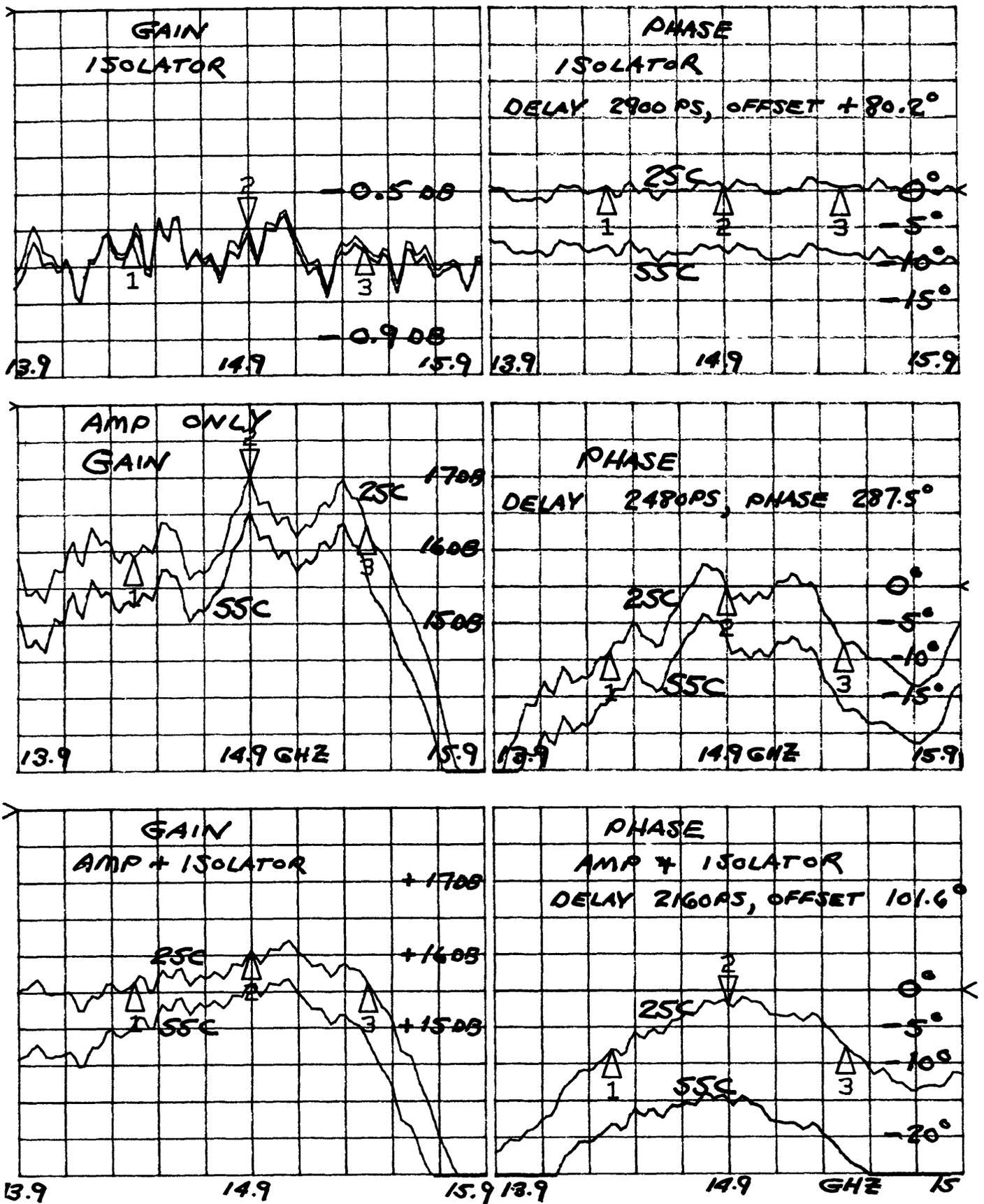
Fig. 4. Test results for KU-band isolator and amplifier.
