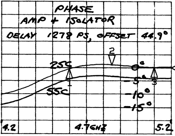
Fig. 2. Test results for C-band filter, isolator, and amplifier.
