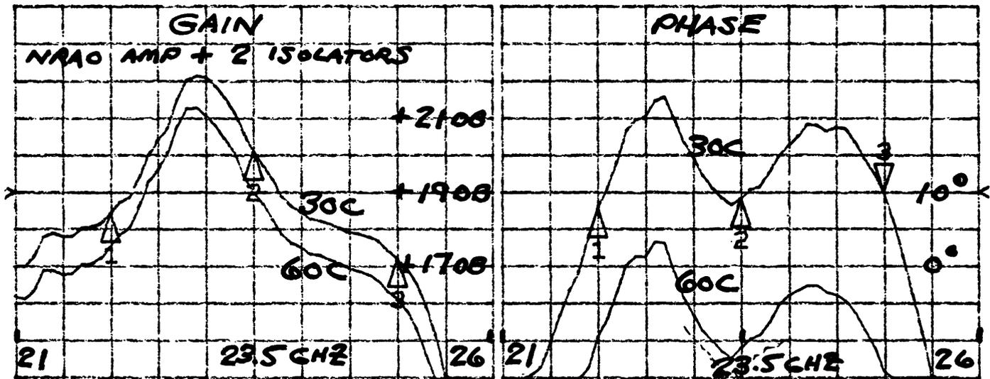
Fig. 5. Test results for K-band isolators and amplifier.
