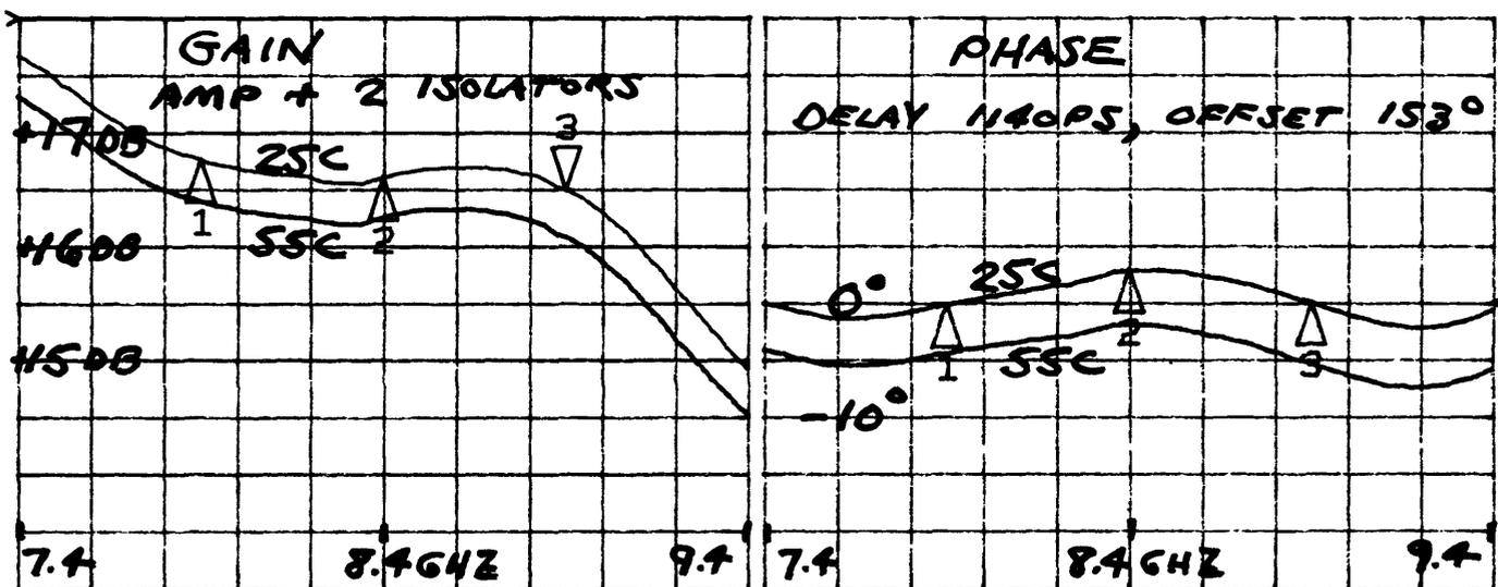
Fig. 3. Test results for X-band isolators and amplifier.
