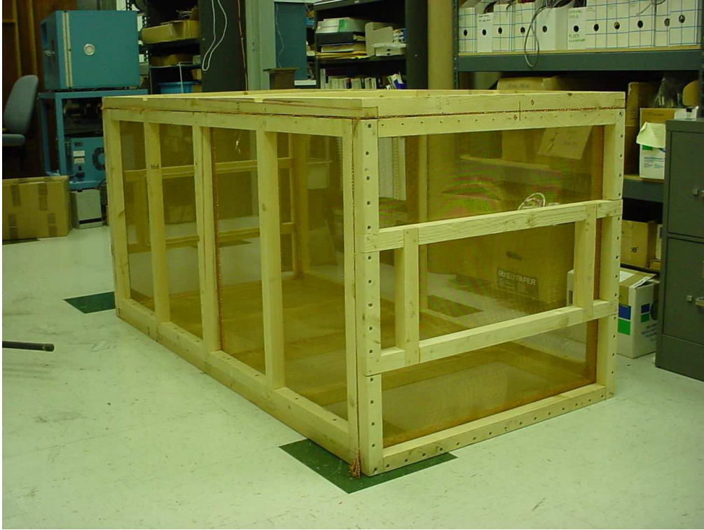
Figure 1. Photograph of the shielded enclosure. The top cover is removable. The wooden framework for one of the bulkheads is visible on the end.
