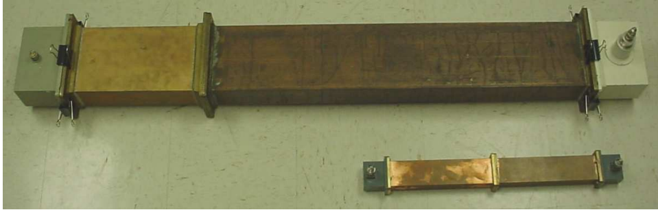
Figure 5. Photograph of the two waveguide test fixtures for measuring the transmission through the screen. The larger one is for 1.5 GHz and the smaller for 3.5 GHz.
