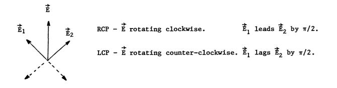
When  $\vec{E}_1$  and  $\vec{E}_2$  are brought into time phase,  $\vec{E}$  ceases to rotate, i.e.,  $\vec{E}$  becomes linearly polarized by  $\pi/4$  to  $\vec{E}_1$  and  $\vec{E}_2$ .
