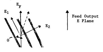
(a)  $\vec{E}_1$  and  $\vec{E}_2$  are in time phase for the desired polarization sense. Then:  $E_F = |\vec{E}_1| \cos \theta + |\vec{E}_2| \sin \theta$
