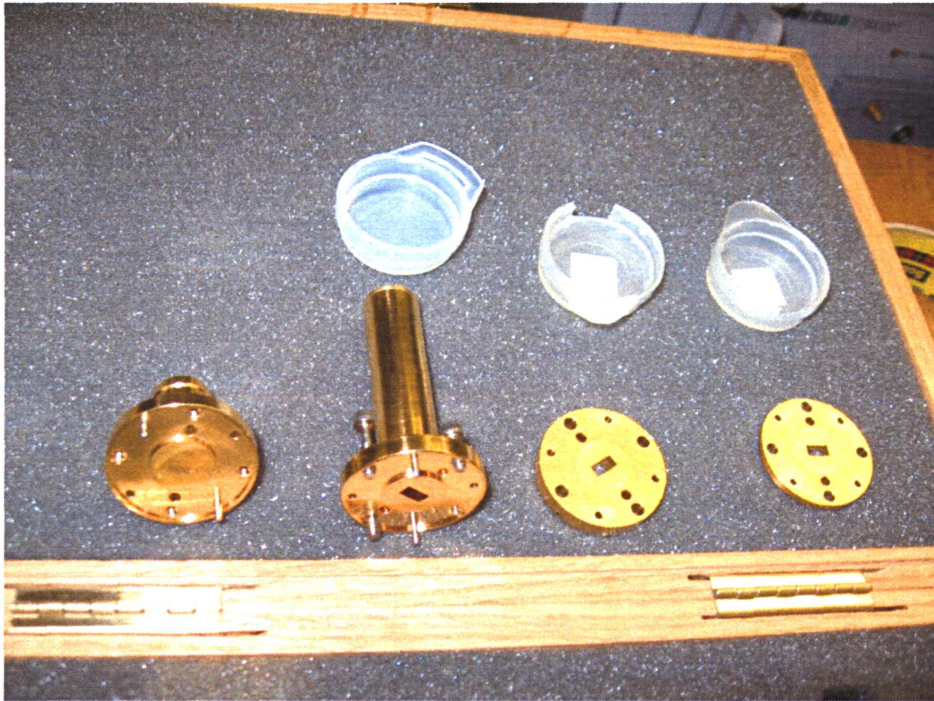
Figure 3: Q-band cal kit: Short, termination, 4.9644mm offset short, 2.5438mm offset short
