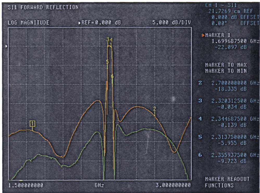
Figure 10: Orange – BSF2 S11 data. Green BSF1 data. Both at 17K.
