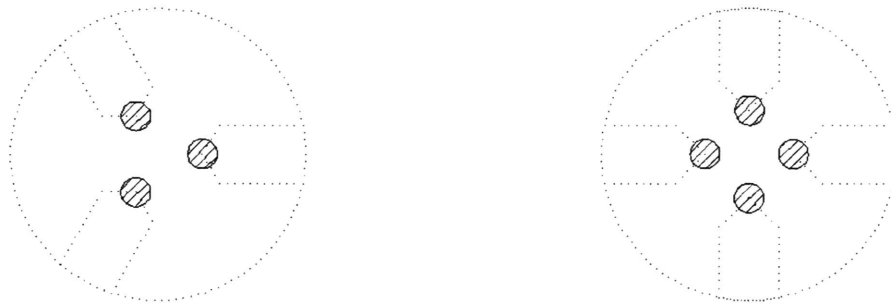
Fig. 8. N -wire model for the low-order modes in ridged waveguides.
