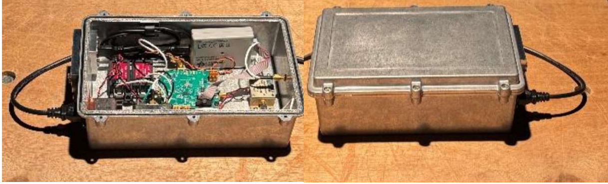
Figure 6. Photograph of the LO module with and without cover. 2
