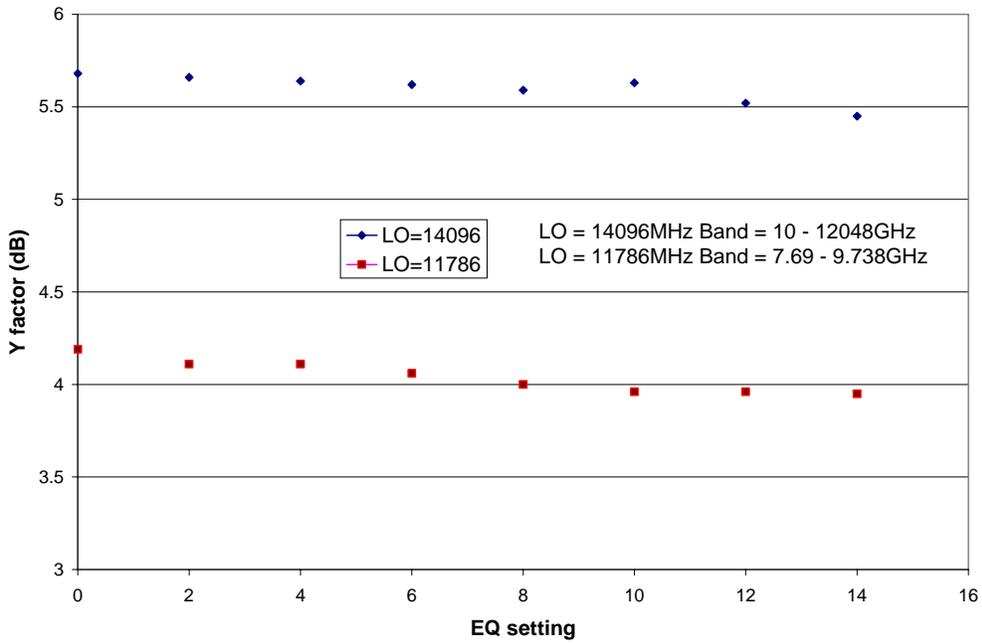
Figure 8: Wideband Y-factor measured at T304 output after proper LO frequency selection allowed viewing of flat regions of UX Converter output spectrum.
