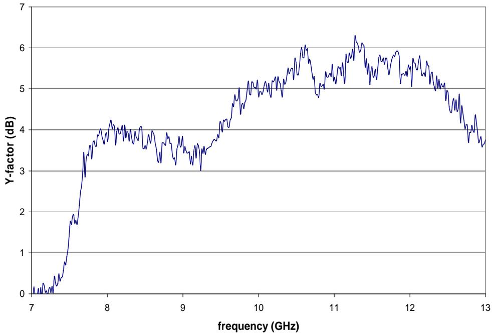
Figure 7: Instantaneous Y-factor at UX Converter output.
