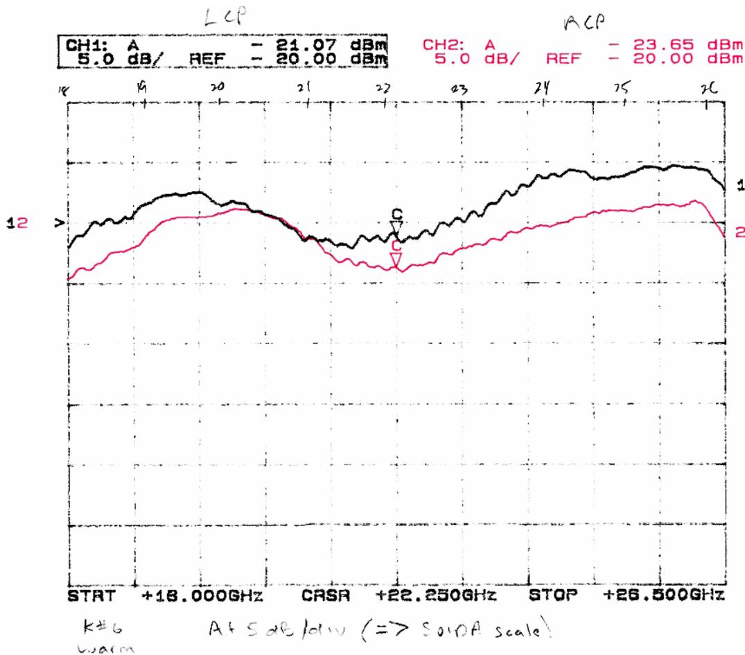
Figure 1: Normalized receiver output spectrum. Vertical scale is 5dB per division.
