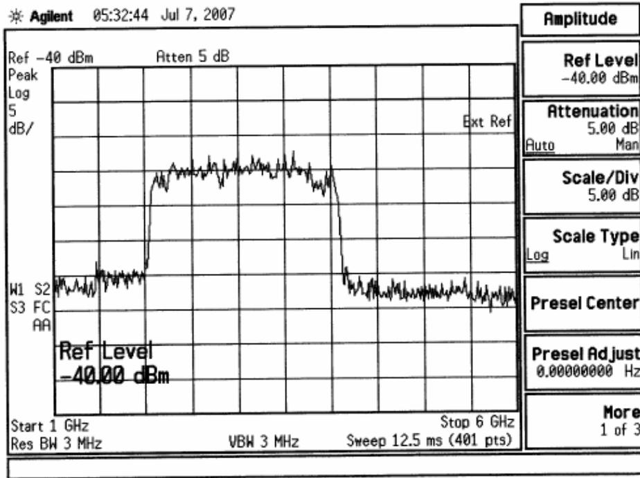
Figure 2: Spectrum analyzer display showing the output passband with no equalizer correction (top), and equalizer correction that yields a maximally flat passband (bottom).
