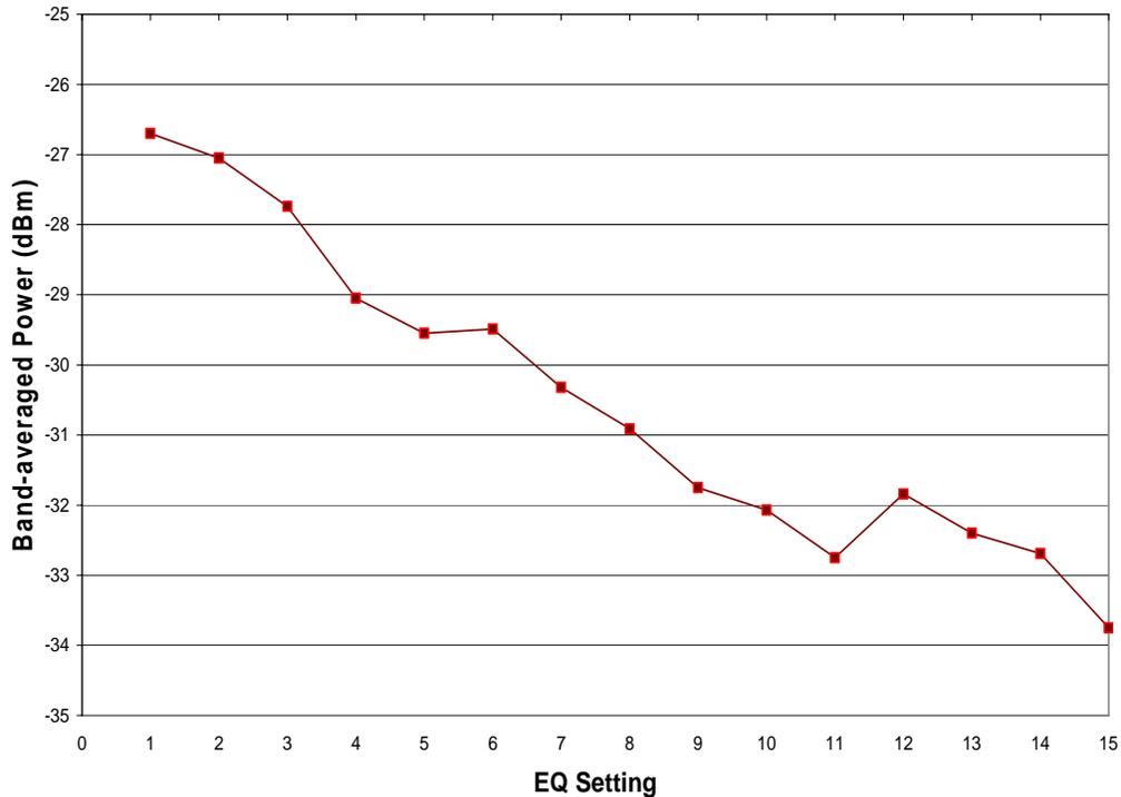
**Figure 4: Band-averaged power versus equalizer setting for the output passband shown in Figure 2. Decreasing power with increasingly positive slope correction indicates that the input signal power was concentrated at the lower end of the spectrum.**
