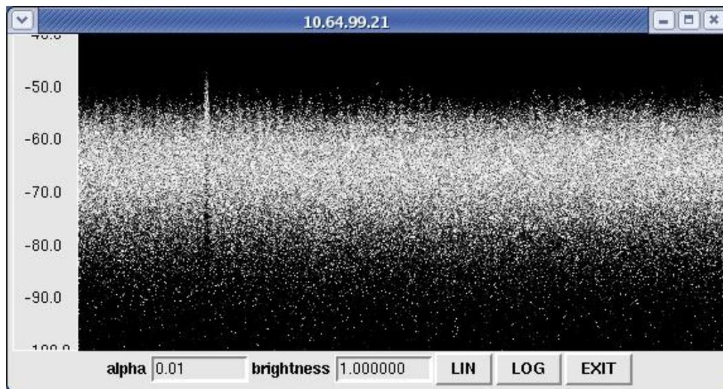
**Figure 3: Digitizer spectral display tool showing sampled 2.048 - 4.096GHz output of T304 with gain slope correction applied. Courtesy: Mike Revnell**
