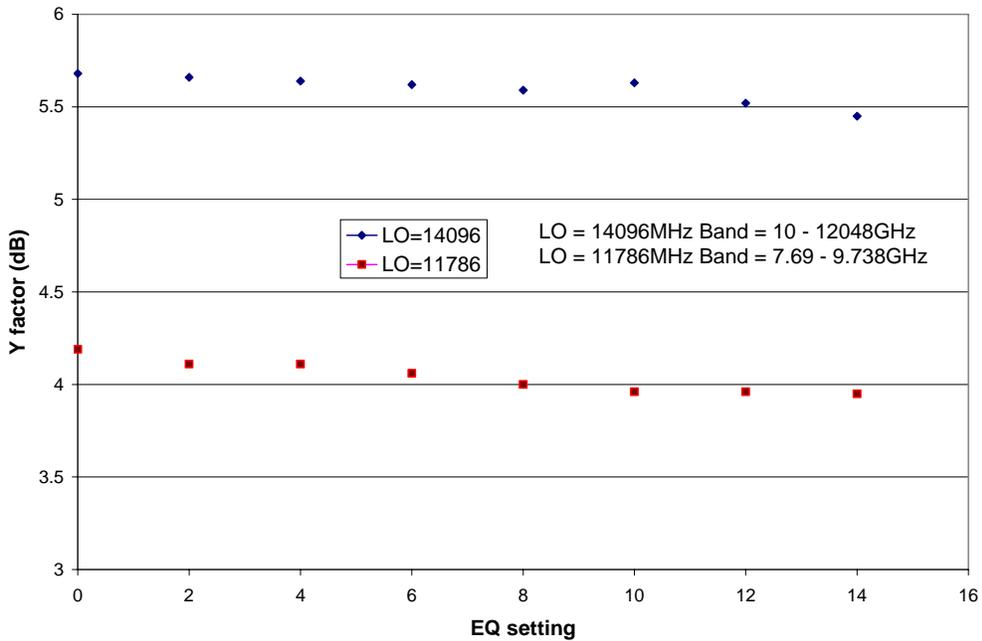
Figure 8: Wideband Y-factor measured at T304 output after proper LO frequency selection allowed viewing of flat regions of UX Converter output spectrum.
