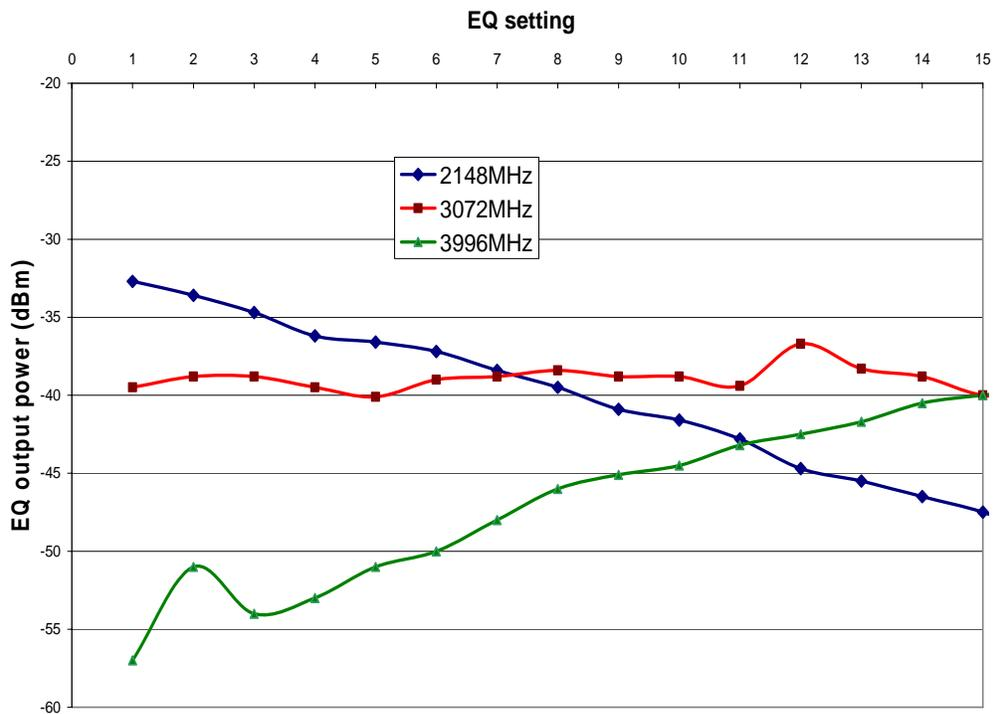
Figure 5: Equalizer response for three sinusoidal signals: 2148MHz, 3072MHz, and 3996MHz.
