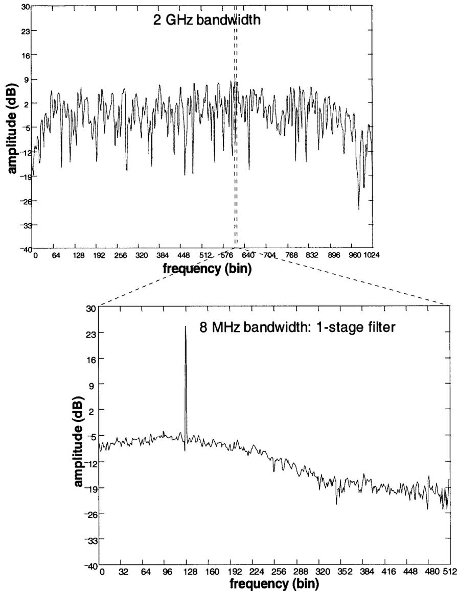
**Figure 2** Simulation of 1/256 narrowband filtering and correlation of a spectrum with lots of structure and a narrowband line. The bands shape has not been corrected and the roll-off at the upper and lower edges of the band is evident (compare this to Figure 4).
