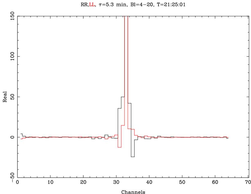
Figure 4: An example of a spectrum showing artifacts around the base of the tone. The apparent tone strength was 2600 and 1400 Jy in RR and LL correlations.
