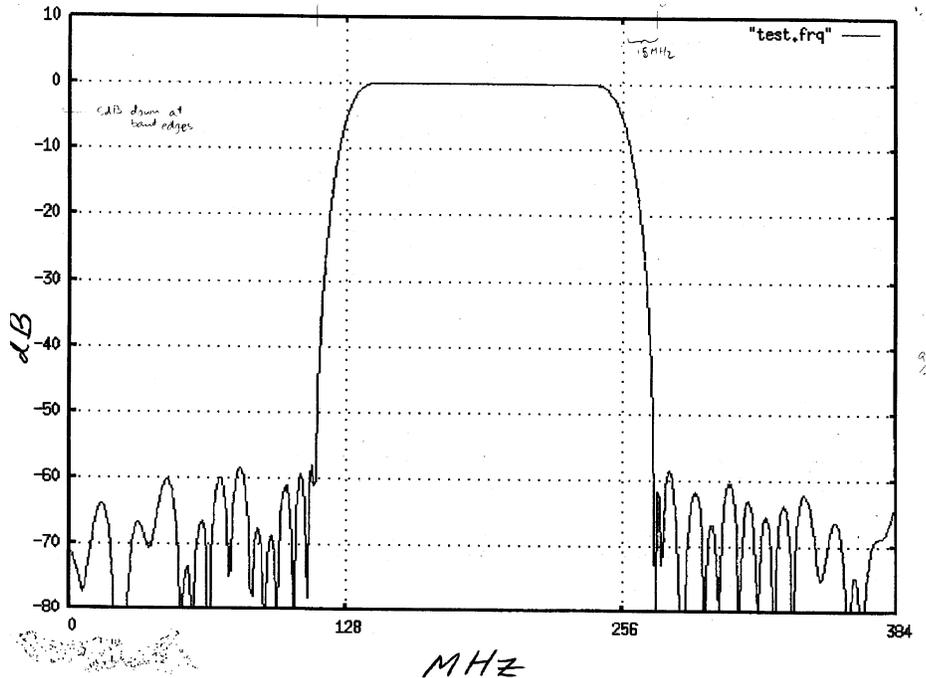
Figure 1: The WIDAR digital filter response of a for a subband bandpass filter. This correctly represents the response after accounting for finite precision arithmetic.
