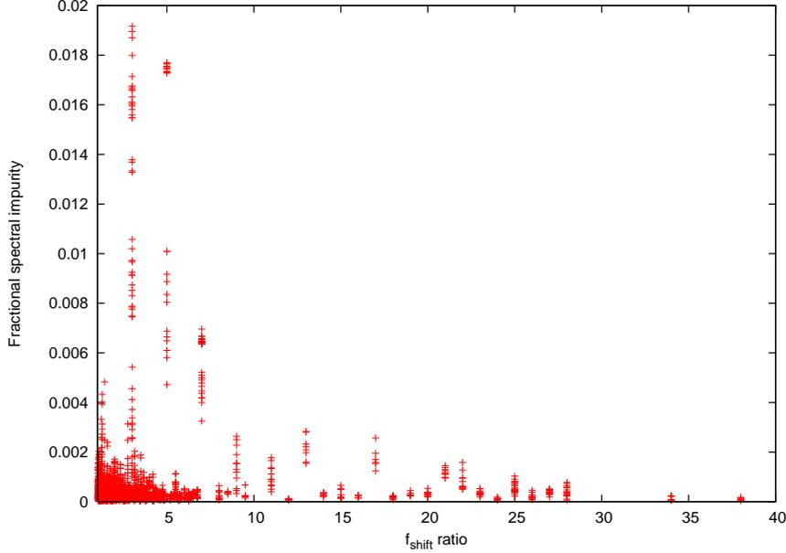
Figure 5: A plot of fractional spectral impurity against  $f_{\text{shift}}$  ratio for frequency configurations A, B and D.
