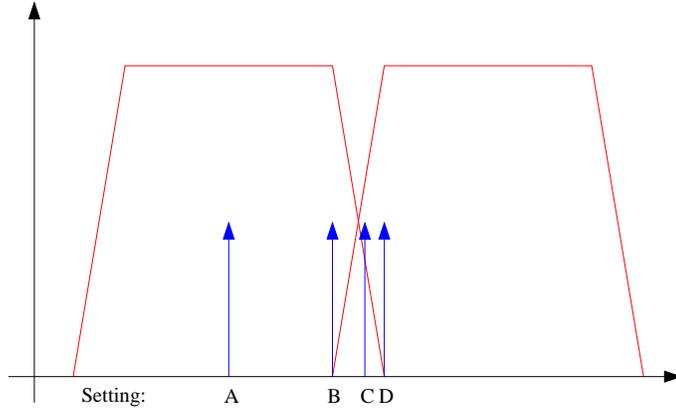
Figure 3: Representation of the location of CW tone within the two observing subbands. The frequency settings of the subbands were varied to place the fixed frequency CW tone at different locations within the passbands.
