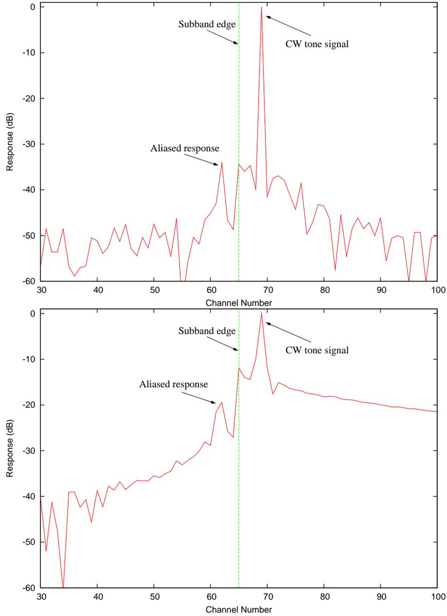
Figure 7: Upper panel: Baseline 7-17 showing an aliased response. The thermal noise floor is near -50 dB. Artifacts approximately 15 dB above this noise floor can be seen around the CW tone. The aliased response is about 35 dB below the tone. Lower panel: Baseline 5-25.  $f_{\text{shift}}$  for antennas 5 and 25 were set to the same frequencies, so there is no fringe washing in reducing the alias response.
