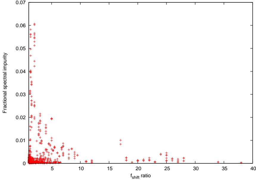
Figure 6: A plot of fractional spectral impurity against  $f_{\text{shift}}$  ratio for frequency setting C.
