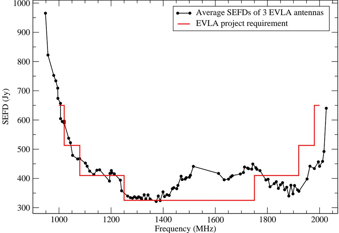
Figure 2: The SEFD values of the EVLA at L-band. No sensitivity measurements are available in the frequency range 1520–1610 MHz, because the data were severely affected by RFI. The red line denotes the EVLA project requirements on the antenna sensitivity at L-band.
