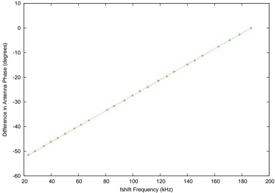
Figure 4: The phase difference in antenna gains, as a function of  $f_{\text{shift}}$ , with and without recirculation. The crosses are the measured difference whereas the line is the expected difference.
