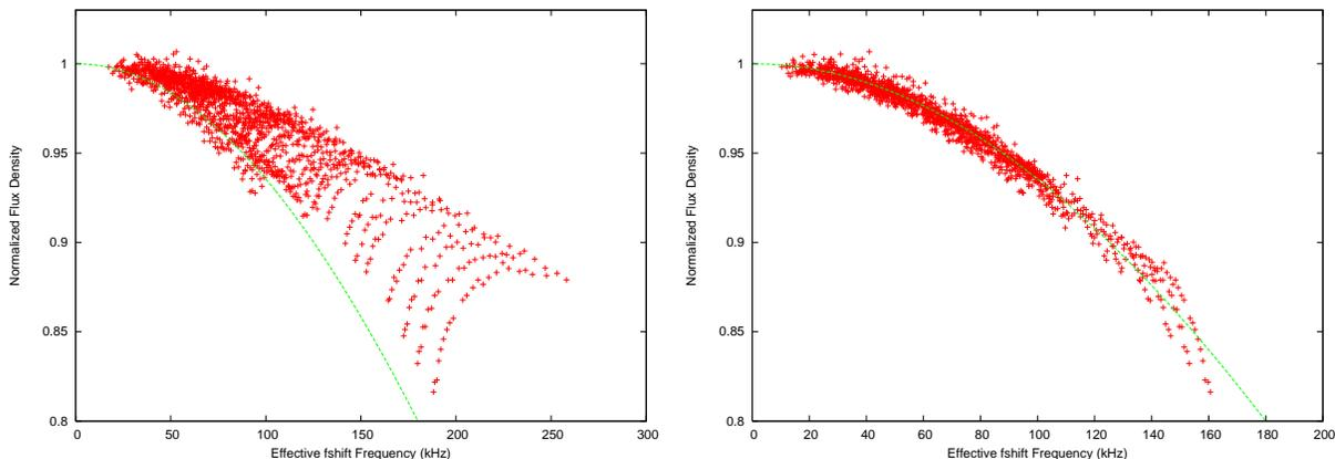
Figure 2: Comparison of predicted (line) and observed (crosses) decorrelation for all test data. The effective phase rate is computed in two different manners. The left panel computes the effective phase rate as antenna phase rates combined in quadrature, whereas the right panel uses the empirical relationship  $f' = 0.88f_x - 0.16f_y$ .
