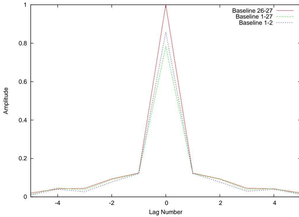
Figure 3: Lag spectra of three baselines showing different amounts of decorrelation with lag number. The  $f_{\text{shift}}$  fundamental for these data is  $f_0 = 6$  kHz.
