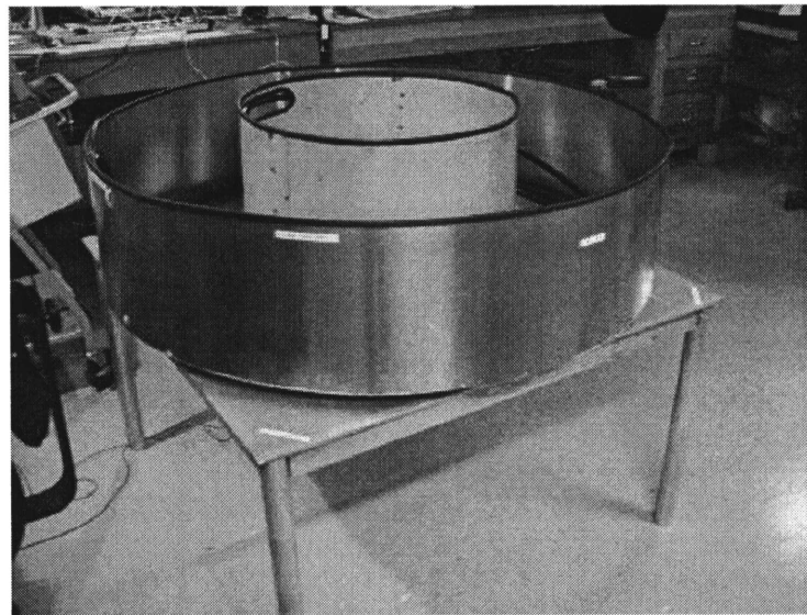
Figure 1, Watch-spring Cable Wrap Test Fixture.
