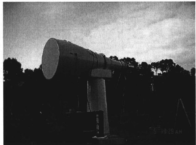
Figure 2. L-Band test setup conducted at Composite Optics, Inc. in San Diego, CA. The foam tower depicted here represents the type of construction that will be used on the OATR.
