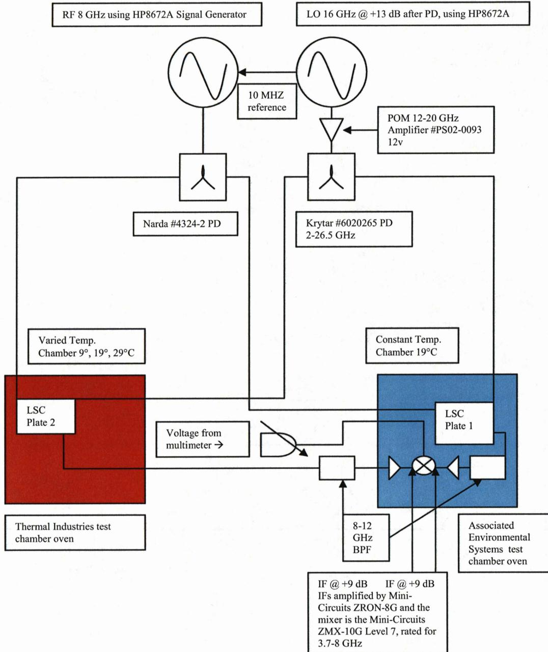
From setup #2, the measured voltages were used to find the upper temperature phase shift and the lower temperature phase shift. Below are the following initial measurements and the follow-up measurements:
