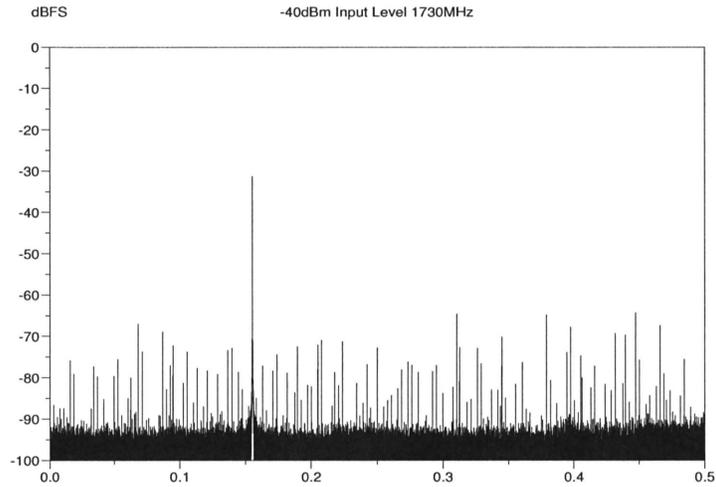
Figure 2 is at the same frequency with the input level increased to just below saturation. The highest spurious signal is around -46 dBFS. This yields ENOB of 7.3 which is consistent with or better than the data sheet specification of 6.5 ENOB.
