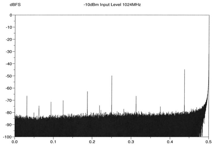
Figure 5 was obtained with the module input terminated at 50 ohms. This represents the noise floor from the digitizer, input amplifiers and crosstalk from other signals inside the module. The highest peak in this plot is below -70dBFS with the bulk of the noise below -90dBFS.
