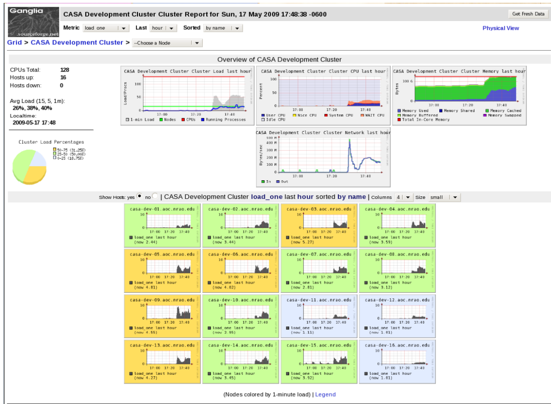
Figure 3: Figure showing a screenshot of the web interface to Ganglia. Top part of the screen shows an overview of the cluster resource usage. The grid of plots in the bottom part of the screen shows the CPU usage as a function of time for each of the 16 nodes.
