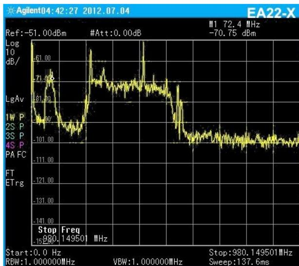
Figure 6 On Antenna: 4/P-band noise powers, 74 MHz -68 dBm; P-band -70 dBm With dipoles, showing noise power now equalized on both bands.
