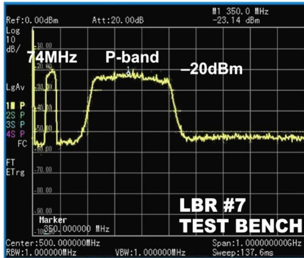
Figure 5 Test bench: Original 4- and P-band noise powers in the lab, 74 MHz set to same total power as P-band. Noise source input -65 dBm.
