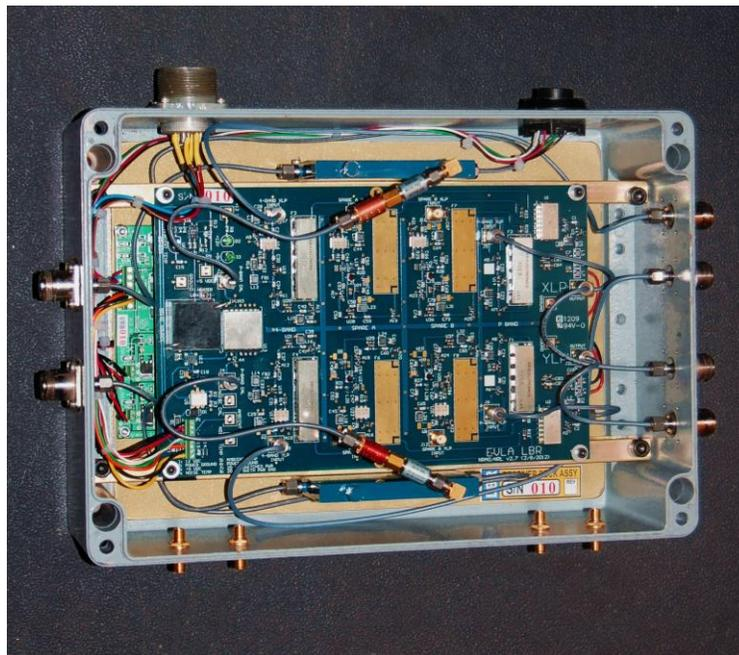
**Figure 1 Photo of an Upgraded Low Band Receiver**
