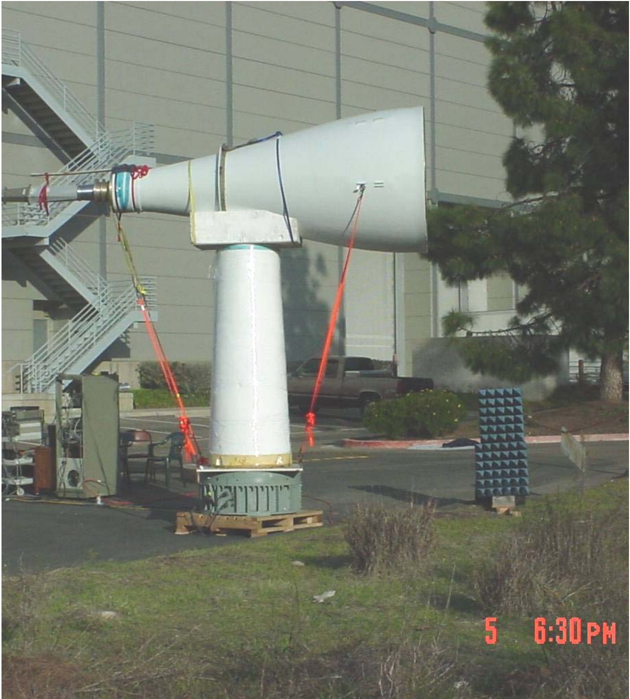
Fig. 11. Feed mounted on azimuth turntable at COI.
