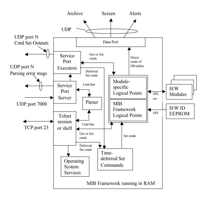
Figure 1. MIB Software Diagram
