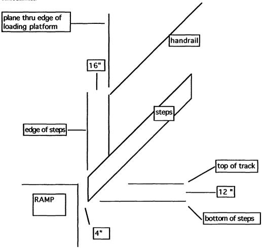
It can be seen that the ramp need be no closer than 20 inches from the face of the loading platfrom at level 1, in order to permit a truck to back up to the loading platform. This gives clearance between all telescope rotating structures and the ramp.
