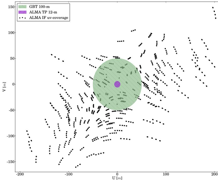
Figure 1:  $uv$ -coverage of the ALMA 12m+7m array for the data used in this memo with the GBT (green) and ALMA TP (purple) coverages overlaid. The GBT data has significant overlap with the ALMA 12-m array  $uv$ -coverage.
